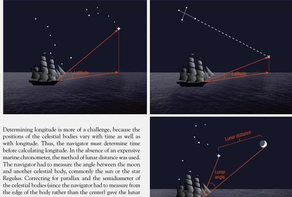
distance, which varied with time. An almanac gave the time in Greenwich, where longitude = 0, for a given lunar measurement. This was compared with the apparent solar time, which could be estimated by the altitude of the sun or a star. The difference in time was multiplied by 15° per hour (the Earth's rotational rate) to give the navigator's longitude.
