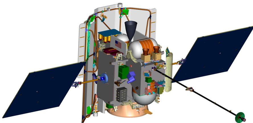
**Figure 2.** The solar panels on MESSENGER could be tilted inward of 0.7 AU from the Sun to reduce the thermal input while still producing sufficient power for the spacecraft.
