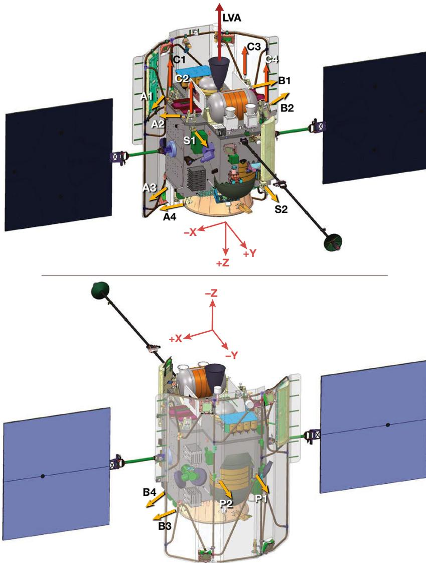
**Figure 9.** MESSENGER thruster locations and exhaust vectors.
