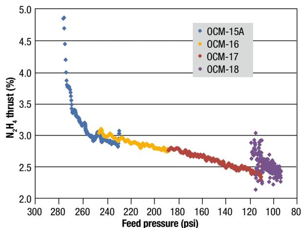
**Figure 11.** Delivered GHe thrust as a percentage of nominal MR-106E hydrazine thrust.
