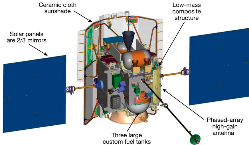
**Figure 1.** Key enabling technologies for MESSENGER.
