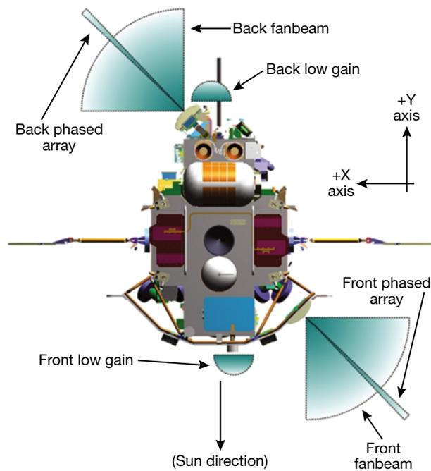
**Figure 4.** The MESSENGER spacecraft antenna suite. The PAA electronically scans  $\pm 60^\circ$  from its boresight in the plane of the figure.
