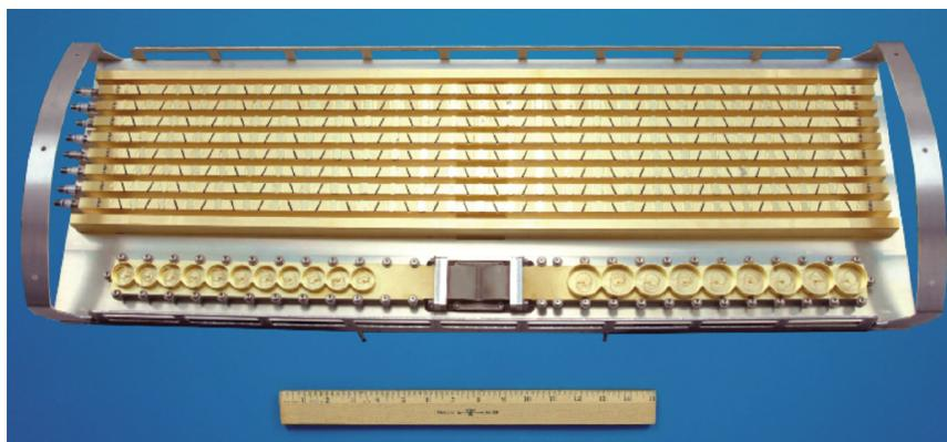
**Figure 3.** MESSENGER phased-array antenna. The upper portion shows the eight slotted waveguides. The lower portion is the medium-gain fan-beam antenna for emergency operations.
