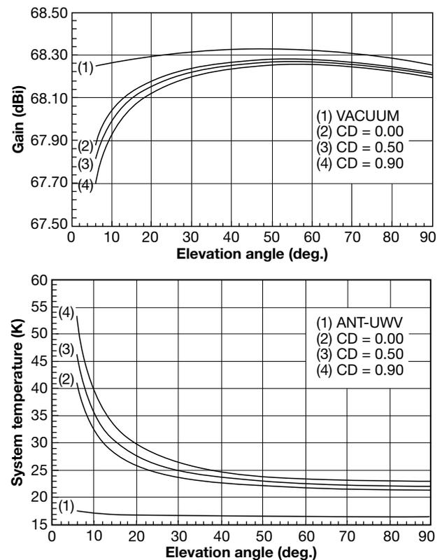
**Figure 5.** DSN ground station performance as a function of elevation angle. ANT-UWV is the antenna performance without weather. The CD traces are the cumulative distribution of effects of 0%, 50%, and 90% weather. (Reprinted with permission from Ref. 12, © 2015, NASA Jet Propulsion Laboratory.)
