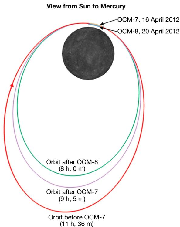
**Figure 7.** Maneuvers OCM-7 and OCM-8 lowered MESSENGER's orbital period from 12 to 8 h.
