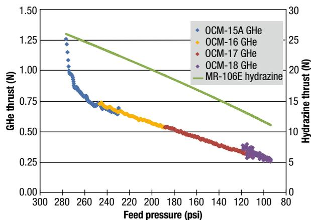
**Figure 10.** Thrust data from all four 22-N nominal MR-106E  $\Delta V$  maneuvers using GHe propellant. Equivalent hydrazine thrust is plotted for comparison.
