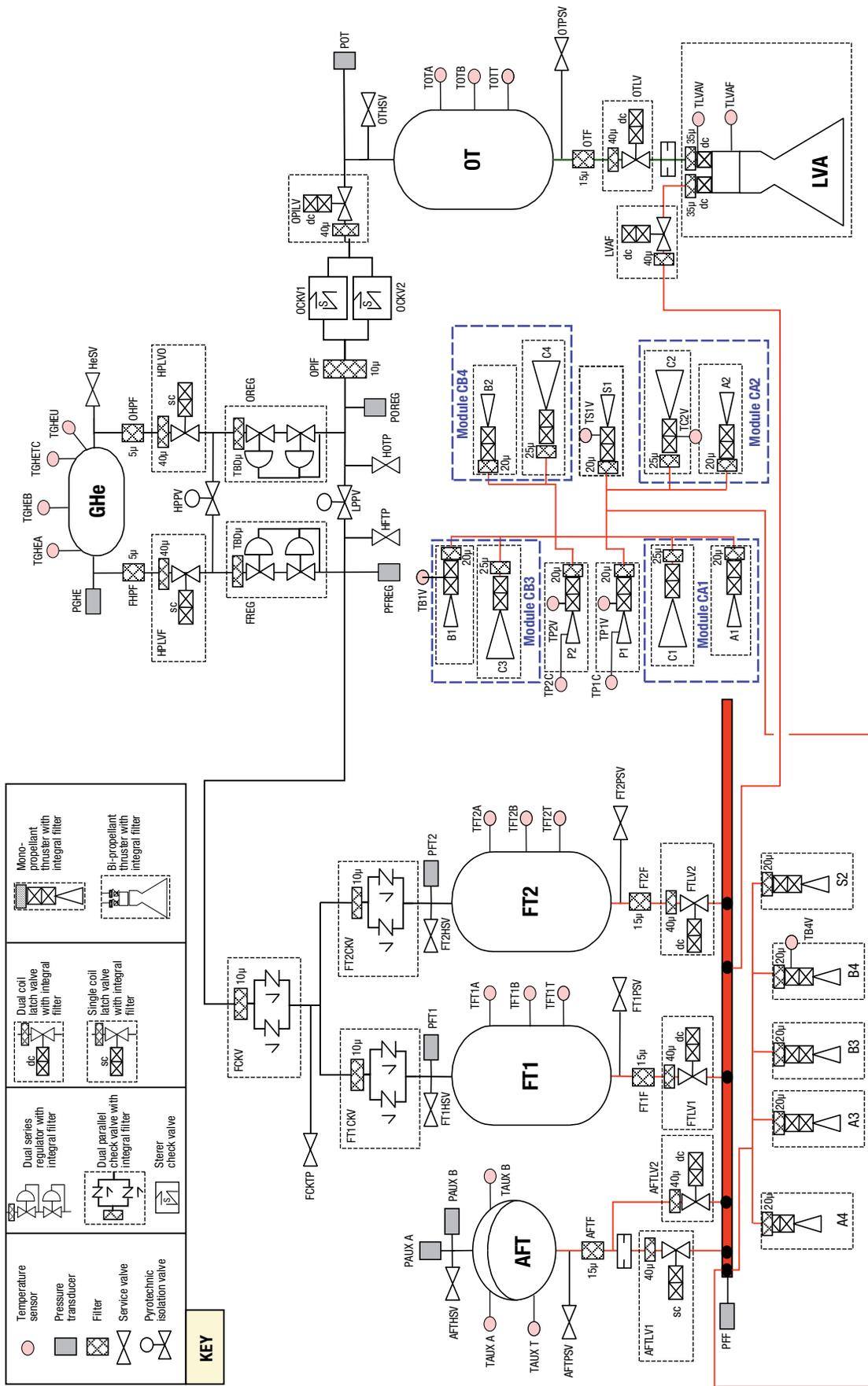
**Figure 8.** Schematic diagram of the MPS. Propellant valves on monoprop thrusters B1, B4, C2, S1, P1, and P2 were instrumented with thermocouples. Owing to their location on the spacecraft sunshade, thrusters P1 and P2 also baselined platinum resistance temperature detectors (RTDs) on their catalyst beds. AFT, auxiliary fuel tank; GHe, helium pressure tank; OT, oxidizer tank.
