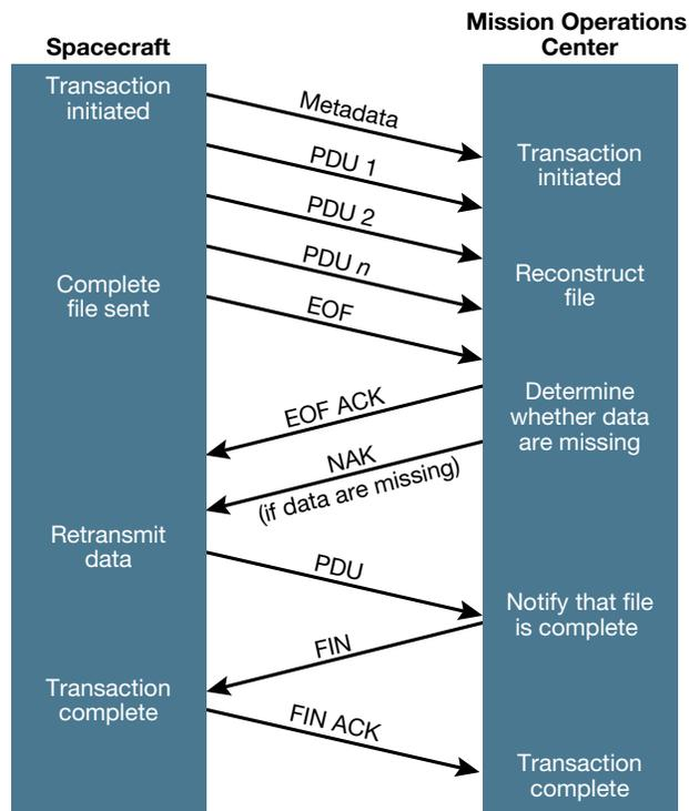
**Figure 6.** An example downlink file transfer with CFDP. ACK, acknowledgment; EOF, end of file; FIN, finished directive; NAK, negative acknowledgment.
