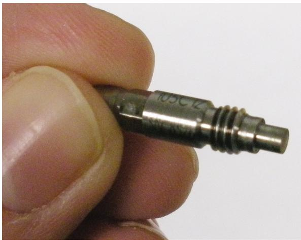
**Figure 16.** The PCB 105C22 dynamic pressure sensor.
