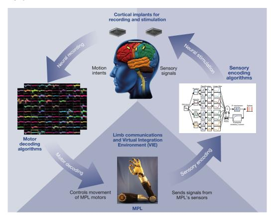
Figure 2. Notional system architecture.
