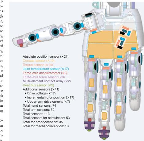
**Figure 4.** The MPL includes more than 100 sensors used for control of the limb and feedback to the MPL user.
