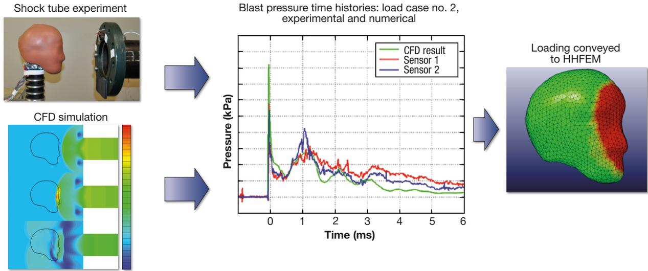
**Figure 4.** Method for establishing the loading inputs to the HHFEM. The experimental conditions for the HSHM are used to validate the results of the computational fluid dynamics (CFD) simulation. After validation, the loads are conveyed to the HHFEM.
