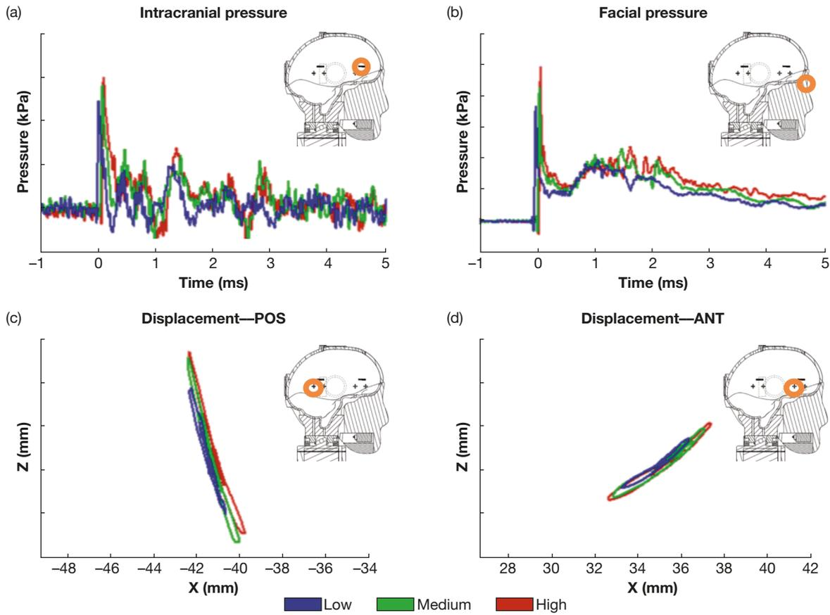
**Figure 2.** Characteristic pressure and displacement data recorded for three test conditions representing (a) the surrogate intracranial pressure, (b) the pressure on the surrogate face, and (c and d) spatial representations of brain motion relative to the skull. POS, posterior sensor; ANT, anterior sensor.
