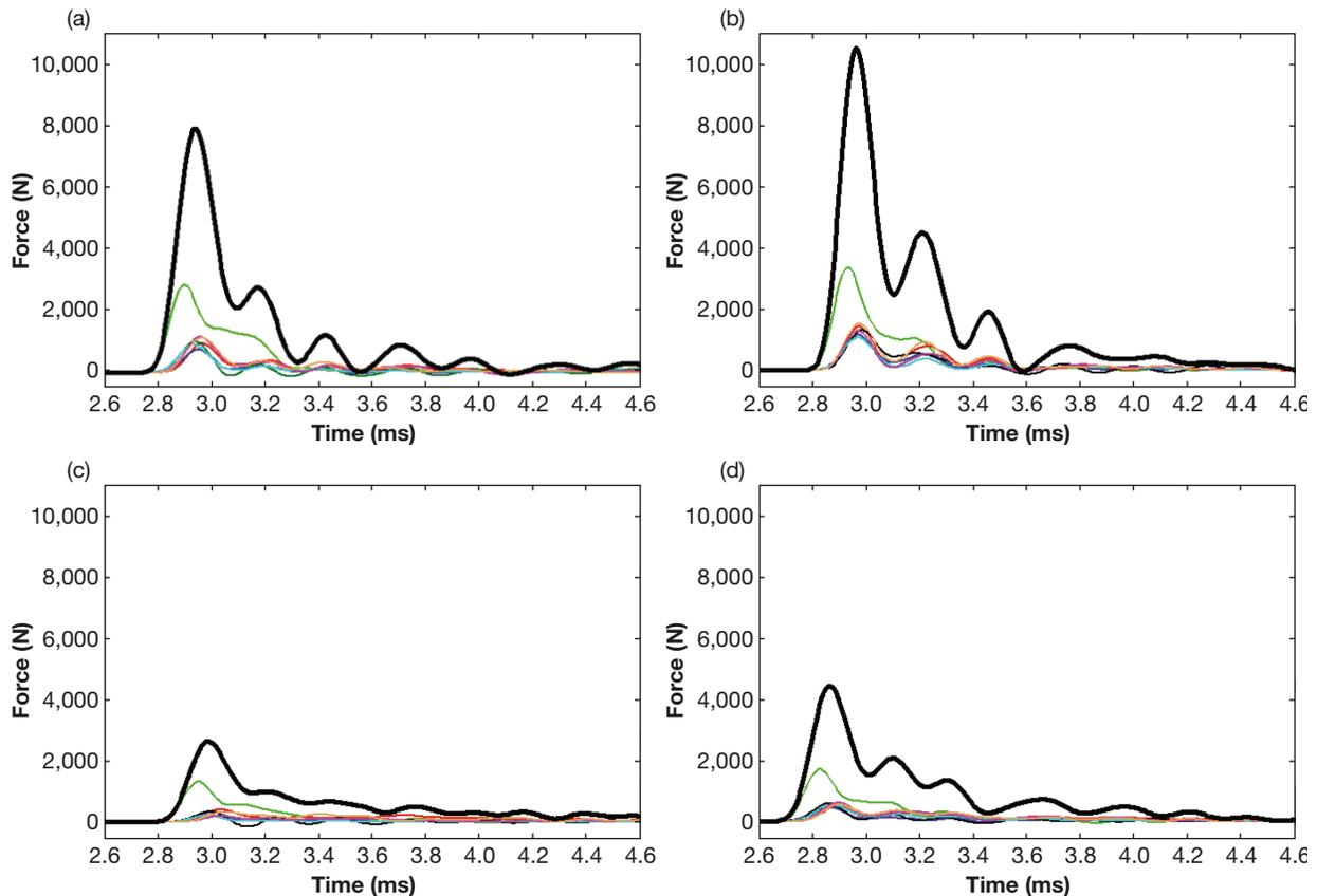
**Figure 9.** Typical force versus time traces for (a) 9-mm FMJ off-pad, (b) 9-mm FMJ on-pad, (c) 4-g RCC off-pad, and (d) 4-g RCC on-pad frontal impacts.
