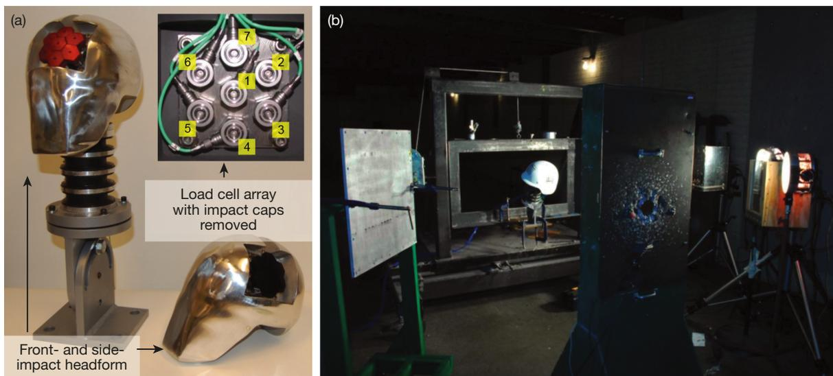
**Figure 8.** (a) Ballistic Load Sensing Headform including load cell array and pivoting base (courtesy of Biokinetics) and (b) behind-helmet blunt trauma ballistics.
