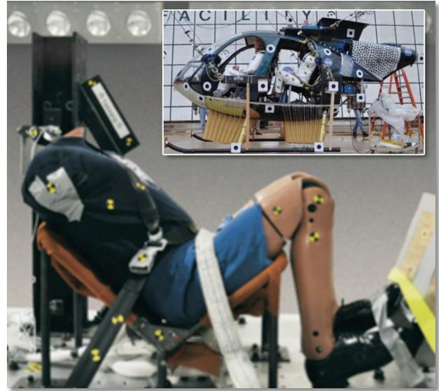
**Figure 10.** Pre-test MD-500 helicopter with installed deployable energy absorber developed by NASA (inset) and laboratory simulation of the helicopter impact deceleration condition, post test.
