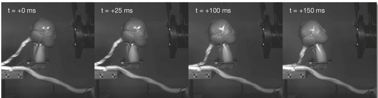
**Figure 3.** Images from high-speed video of a shock tube test (689-kPa driver) on the HSHM.
