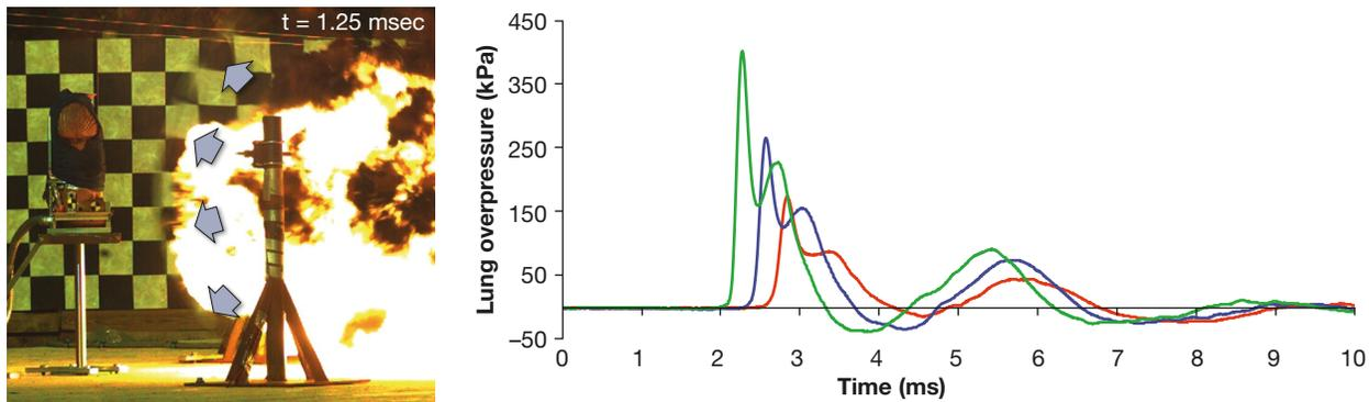
**Figure 7.** Incident shock wave approaching the HSTM during a blast test (left); upon reaching the torso surrogate, instrumentation in the lungs captures the internal overpressure response for three tests of varying charge weights (right).
