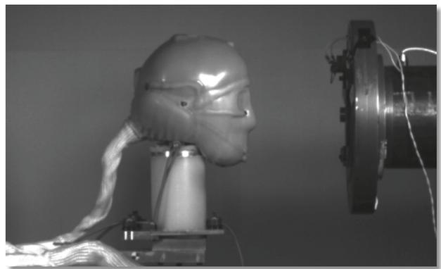
Figure 1. HSHM positioned in front of shock tube.
