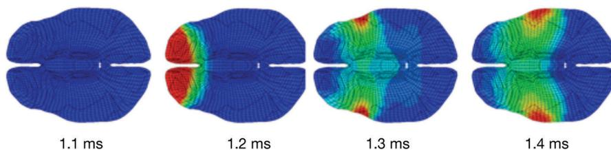
**Figure 5.** Pressure wave propagation response in a transverse plane of the brain of the HHFEM.
