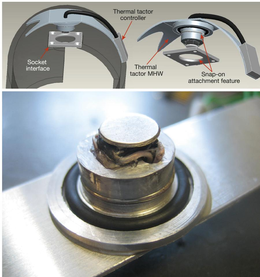
**Figure 4.** (Top) Diagram of the thermal tactor integration with the socket system. (Bottom) The thermal tactor prototype. MHW, mechanical hardware.
