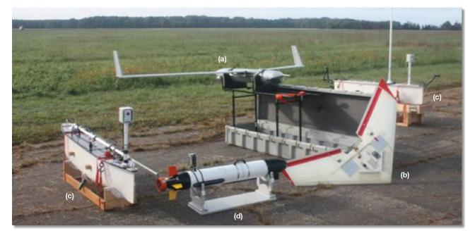
Figure 5. OPISR vehicles featuring (a) ScanEagle, (b) Unicorn, (c) surface vehicles, and (d) Iver2 undersea vehicle.
