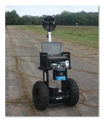
**Figure 6.** OPISR's ground vehicles were Segway RMP 200s that were fitted with lidar, electro-optic, and passive acoustic sensors.
