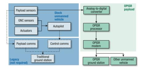
**Figure 3.** OPISR's hardware architecture is based on a modular payload that can be fitted onto different types of unmanned vehicles.
