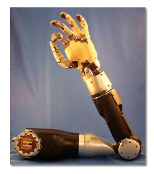
**Figure 1.** This final prototype of the MPL, successfully demonstrated to DARPA in December 2009, offers 22 degrees of freedom.
