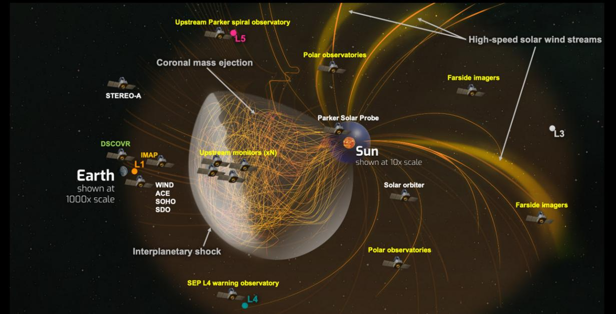
Solar transients are both immense and highly complex magnetic structures. The magnetic field lines shown in this graphic are based on a physics-based simulation using the Grid Agnostic MHD for Extended Research Applications (GAMERA) model. The vast size difference between Earth and transients requires a multiscale measurement approach to capture the information necessary for successful and actionable space weather prediction. Observatories marked in yellow indicate identified observation gaps.
