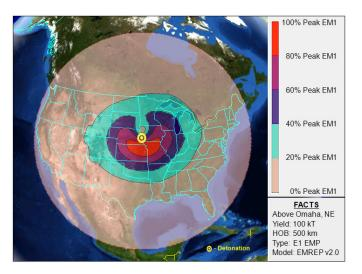
EMP coverage area on the ground increases as the height of the burst increases. A nuclear detonation at an altitude of five hundred kilometers over Omaha, Nebraska, will generate an EMP that covers the contiguous land mass of the United States. The electric field strength diminishes with increased distance from ground zero directly under the burst. The asymmetry in contours is a result of the orientation of Earth's magnetic field with respect to the detonation point.
