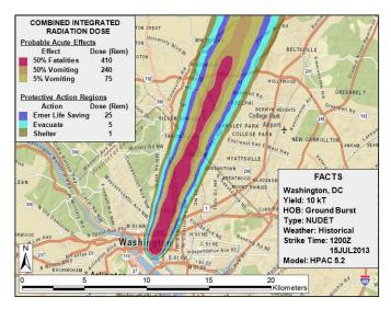
Depicted are the bands of varying fallout contamination as predicted by the Hazard Prediction Assessment Code (HPAC). Each color contour represents the cumulative dose that would be seen by a sensor situated at that location from the time of detonation. Because many fission products decay rapidly, a sensor introduced at later times would accumulate a significantly lower total dose.
