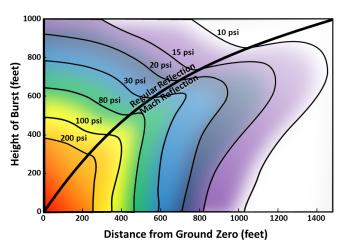
In the Mach reflection region, the incident and reflected shock waves have merged to form a single shock front called the Mach stem. Extended knees in the Mach reflection region, more prominent at overpressure levels below one hundred pounds per square inch, make air bursts more effective for maximum overpressure damage to structures and other ground targets.<sup>51</sup>
