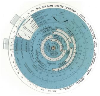
Previously provided as a supplement to Glasstone and Dolan's classic *Effects of Nuclear Weapons*, this shirt pocket slide rule calculator was widely used in the 1950s–1970s but has now been replaced by digital computational resources that use fast-running predictive codes and algorithms.
