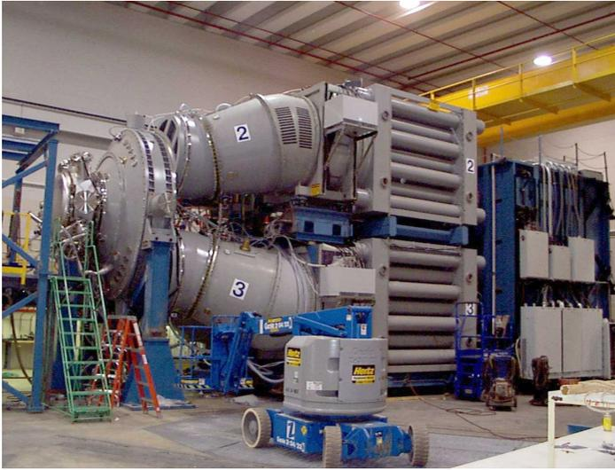
**Figure 6.5. DECADE X-Ray Simulator Module.** This photograph shows the first of four pulsed power modules planned for the DECADE simulator. The simulator was never completed, a victim of post–Cold War apathy and budgetary declines visited on all matters nuclear. A similar fate eventually befell many other nuclear effects simulators. (Image courtesy of the Department of Defense.)
