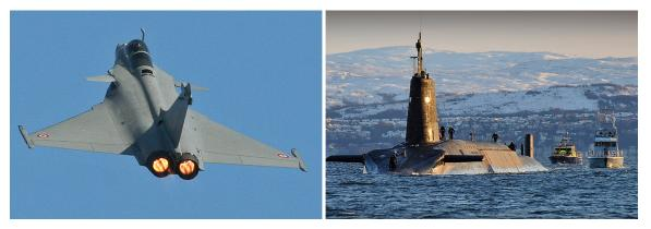
The French Dassault Rafale C multi-role fighter (left) is capable of carrying the nuclear ASMP-A, an air-tosurface, ramjet-powered, inertially guided supersonic standoff missile with a reported range of hundreds of kilometers. The United Kingdom's *Vanguard*-class submarines are capable of launching Trident II nuclear ballistic missiles. Shown here is HMS *Vanguard* (right) entering Faslane Bay, Scotland, where all four boats are based at Her Majesty's Naval Base Clyde.
