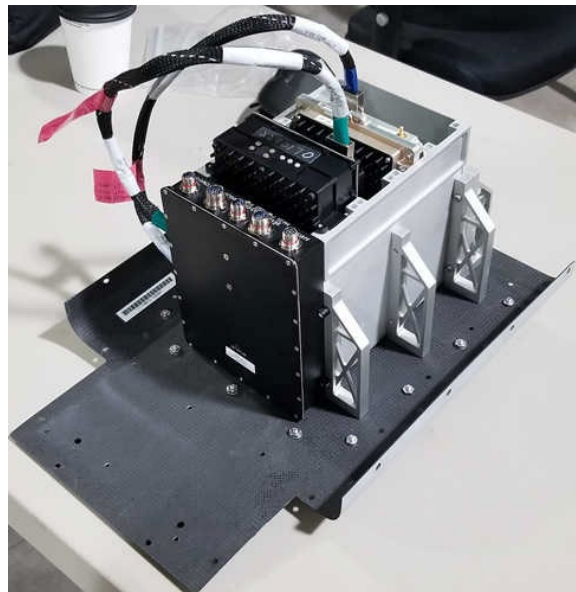
Figure 4-52. Jump-20 Primary Mount with MAIM and Two Payloads
