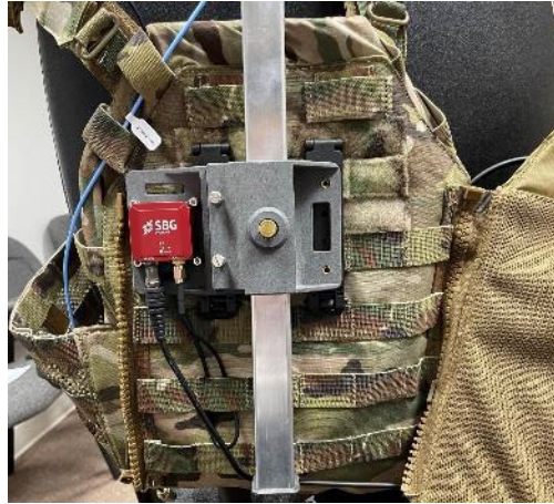
Figure 4-167. Mast-mounted INS Location
