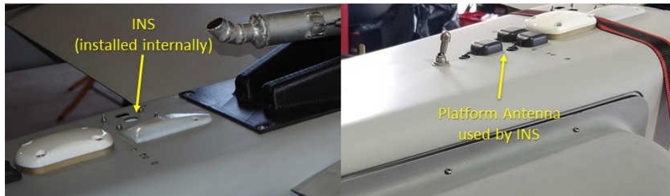
Figure 4-56. Jump-20 INS Location and GPS Antenna
