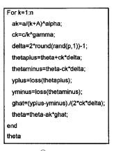
Fig. 1. Sample MATLAB® Code for SPSA. (Initialization for program variables theta, n, p, a, A, c, alpha, and gamma not shown.)
