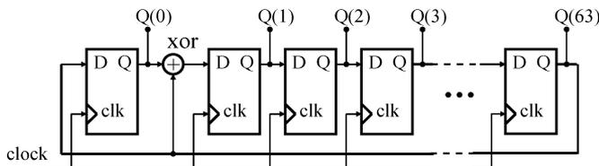
Fig. 7. Configuration of the linear feedback shift register.
