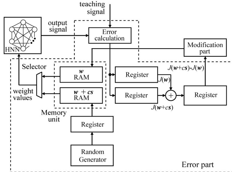
Fig. 6. Configuration of the error part.
