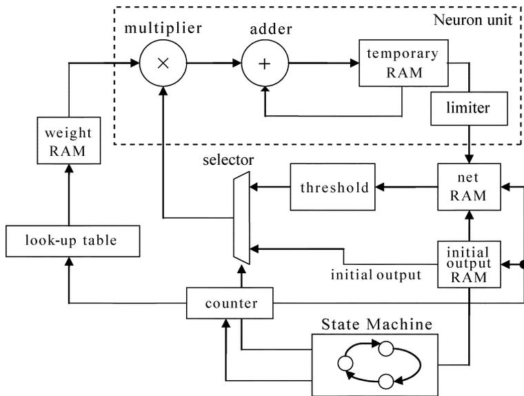
Fig. 9. Configuration of the HNN from arithmetic operation point of view.
