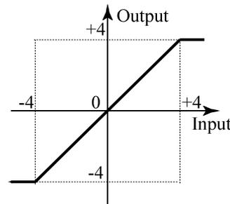
Fig. 5. Input-output characteristics of neurons.
