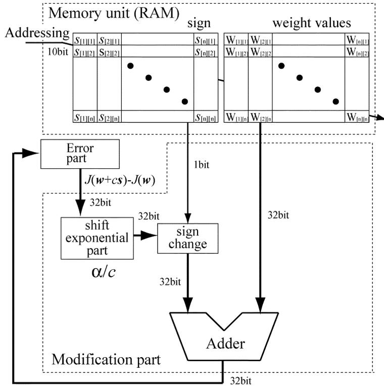
Fig. 8. Configuration of the modification part.
