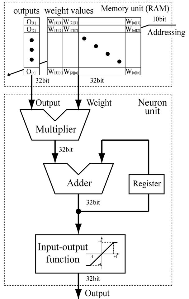
Fig. 4. Configuration of the neuron unit.
