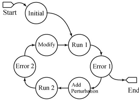
Fig. 3. State flow of the overall HNN system.
