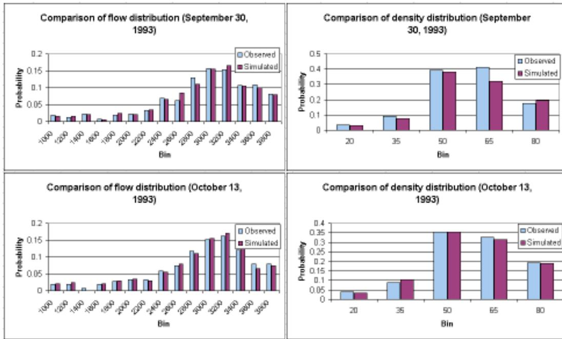
Figure 6 Comparison between simulated and observed flow and density distributions (September 30, 1993, October 13, 1993).
