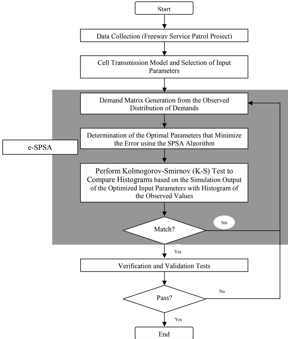
Figure 2 Proposed combined enhanced SPSA simulation calibration methodology.
