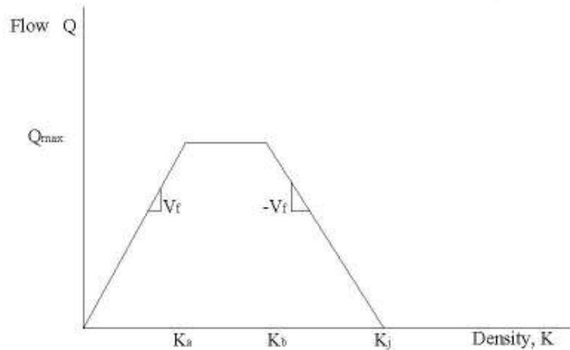
**Figure 1:** Flow-density relationship for the basic cell transmission model [16]
