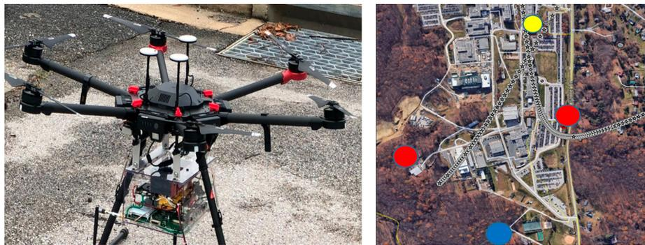
**Figure 6.** Prototype SDR sensor. Left, UAS with integrated ES payload. Right, Time-difference-of-arrival isochrones from two UASs. The Blue node is stationary, the Red node moved between two limited points, and the yellow node is the rooftop radar target.
