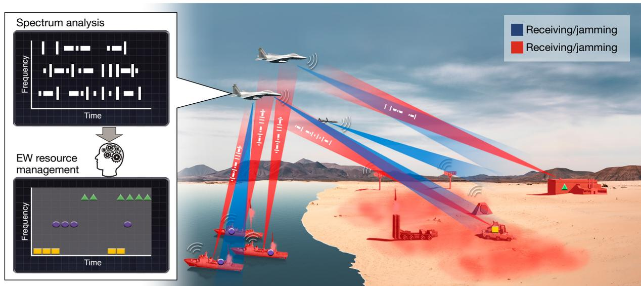
**Figure 3.** Autonomous and adaptive EW concept example. Shown is a single-platform autonomous resource management scenario, where received radar pulses are characterized and linked to specific Red threat systems. The spectrum analysis view shows received radar pulses from three unique threat systems. Once those threat systems are characterized, EW receiver and jamming resources are dynamically organized according to mission constraints and threat system behavior over time.
