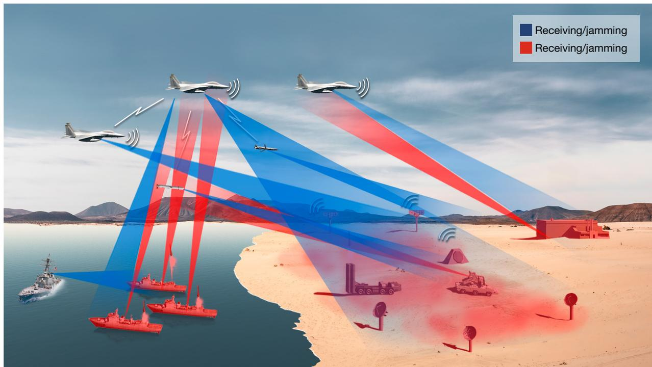
**Figure 4.** Collaborative electronic fires concept example. In this example, notional Blue airborne stand-in, stand-off, and fighter platforms are approaching a Red integrated air defense system and surface action group. In this distributed concept, the stand-in sensor senses target RF emissions and periodically passes this information via a data link to the two stand-off EW systems so that they can update their EA techniques and cover all Red threat systems.
