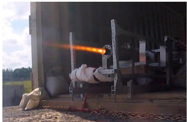
**Figure 16.** Still image of the first 6-s test. This test campaign evaluated the motor's performance and validated the ballistics model. The test duration was set to 6 s, with a 1-s start-up sequence to ensure proper ignition. We chose the start-up transient of 1 s so that enough heat from the igniter would start to pyrolyze the fuel grain while also slowly introducing the oxidizer to ensure the flame would not be blown out.
