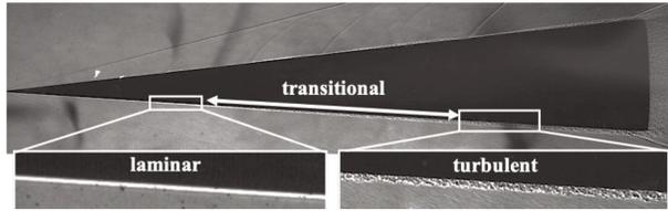
**Figure 1.** Shadowgraph image of boundary-layer transition. This image is over a 5° half-angle sharp cone traveling at Mach = 4.31 in free flight at an aeroballistics range. Labels of boundary-layer states and cropped image insets have been added. (Adapted from Schneider,<sup>5</sup> with permission from Elsevier.)
