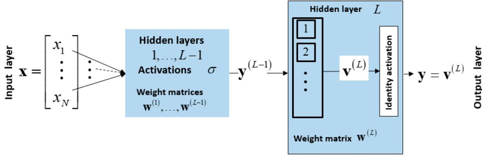
Fig. 10. A fully connected regression neural network with  $L$  hidden layers: the first  $L - 1$  layers have activation  $\sigma$  and weight matrices  $\mathbf{w}^{(1)}, \dots, \mathbf{w}^{(L-1)}$ , and the last hidden layer has weight matrix  $\mathbf{w}^{(L)}$  with identity activation so that  $\mathbf{y} = \mathbf{v}^{(L)}$ .
