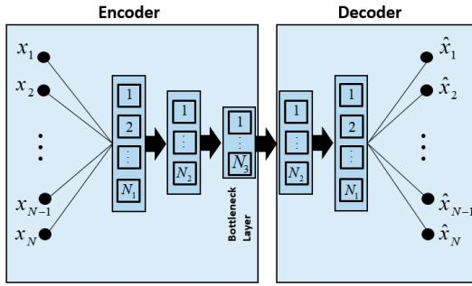
Fig. 37. Basic autoencoder configuration with input  $N \times 1$  data vector. The encoder portion has three hidden layers with  $N_1 > N_2 > N_3$  neurons, with the last hidden layer known as the bottleneck layer. The decoder portion has two hidden layers with  $N_2$  and  $N_1$  neurons, respectively. The output vector has the same dimension  $N$  as the input vector.
