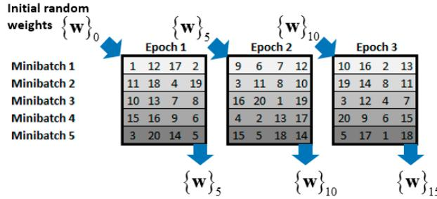
Fig. 14. Example of mini-batch training: training indices  $[1, \dots, 20]$ , mini-batch size of 4, three epochs, resulting in 15 weight updates.
