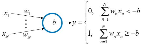
Fig. 4. A threshold computing unit model of a neuron.
