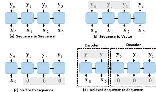
Fig. 33. Different recurrent network architectures.
