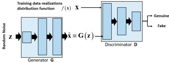
Fig. 38. A typical Generative Adversarial Network (GAN). Each rectangle represents a hidden layer of arbitrary size except for: the output layer of  $\mathbf{G}$  which must match the dimension of  $\mathbf{x}$ , and the output of  $\mathbf{D}$  which must allow for binary classification (i.e., single sigmoid node or two softmax nodes).
