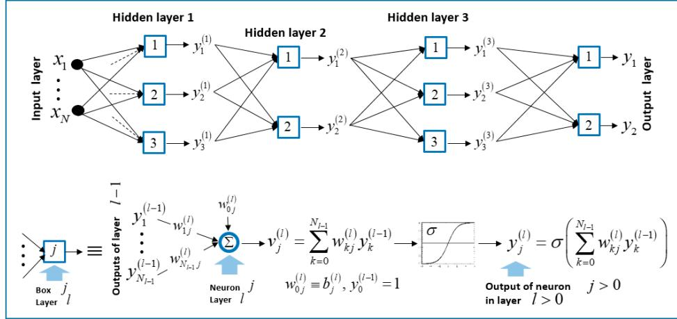
Fig. 8. An artificial neural network  $\mathbf{y} = h(\mathbf{x})$  whose input layer ( $l = 0$ ) has  $N$  elements, three hidden layer ( $l = 1, 2, 3$ ) with 3, 2, 3 neurons, respectively, and an output layer ( $l = 4$ ) with 2 neurons. Each square box in the network represents a neuron shown on the bottom.
