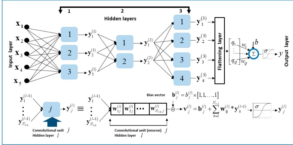
Fig. 16. A CNN with 5 time series of equal length in the input layer, 3 hidden layers, and an output layer with 1 scalar output. The bottom portion describes each convolutional unit (neuron), where  $\mathbf{w} * \mathbf{y}$  indicates correlation between the two sequences  $\mathbf{w}$  and  $\mathbf{y}$ . The flattening layer in this example produces 1 scalar output for a 2-class classification network.
