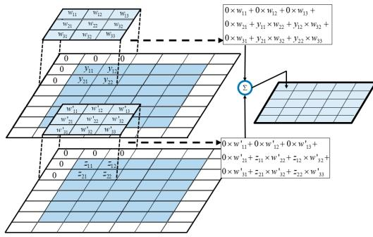
Fig. 19. Zero padding  $5 \times 5$  images and correlating with two  $3 \times 3$  filter matrices.
