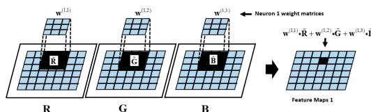
Fig. 21. Feature map 1 generated from stride 1 sliding correlation values obtained by sum of dot products of neuron 1 weight matrices with correspondingly aligned  $3 \times 3$  image sections (white sections around RGB images indicate zero padding).
