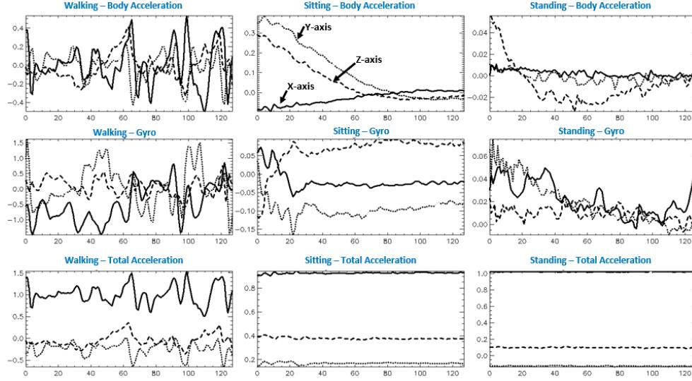
Fig. 22. Vector time series (three spatial axes) for three of six activities of the HAR data from UC Irvine: body acceleration, gyro, and total acceleration for Walking, Sitting, and Standing.
