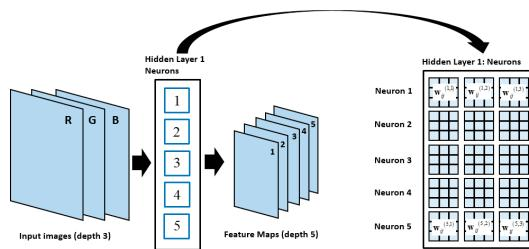
Fig. 20. Input layer images with depth 3, first hidden layer with 5 convolutional neurons, and 5 feature maps - box on the right shows a detailed picture of all the weight matrices for all 5 neurons.
