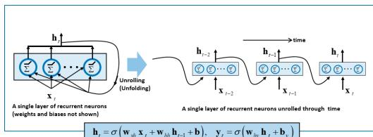
Fig. 32. A layer of recurrent neurons and its unrolling through time.
