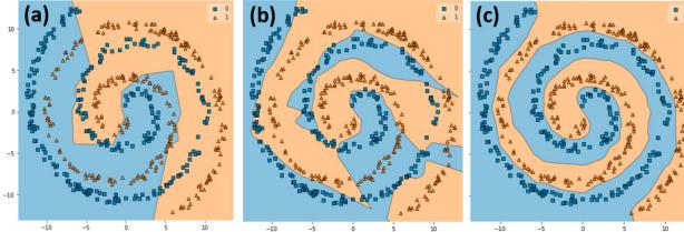
Fig. 12. Classification boundaries for three neural networks with a single hidden layer and 10 (a), 1000 (b), and 5000 (c) neurons, respectively.
