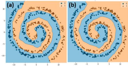
Fig. 13. Classification boundaries for two neural networks with 2 (a) and 3 (b) hidden layers, each with 10 neurons.
