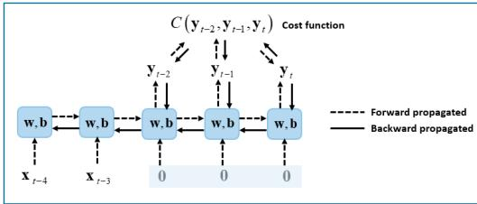
Fig. 34. Data flow for backpropagation training of an RNN.
