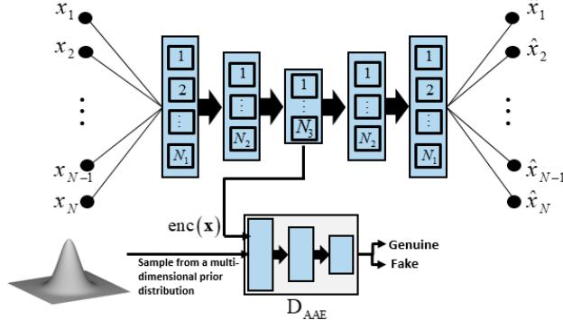
Fig. 40. Adversarial Autoencoder (AAE): an autoencoder coupled with a discriminator, trained using the same alternating phases as GANs.
