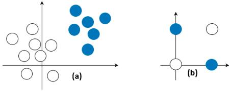
Fig. 7. Pattern (a) shows linear separation; no straight line can separate the pattern in (b).
