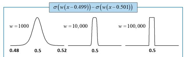
Fig. 3. The difference between two sigmoid functions  $\sigma(w(x - s + 0.001)) - \sigma(w(x - s - 0.001))$  for  $s = 0.5$ ,  $w = 1000, 10,000, 100,000$ , for  $x \in [0.48, 0.52]$ .
