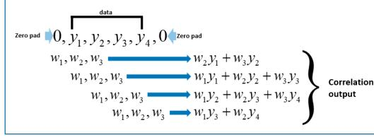
Fig. 17. Correlation procedure for an input sequence with 4 elements and a filter with 3 elements, resulting in an output with 4 elements.
