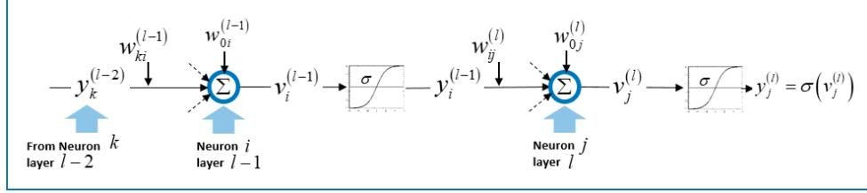
Fig. 9. A portion of a feed forward neural network:  $y_k^{(l-2)}$  is the output of neuron  $k$  in layer  $l - 2$ ,  $y_i^{(l-1)}$  is the output of neuron  $i$  in layer  $l - 1$ , and  $y_j^{(l)}$  is the output of neuron  $j$  in layer  $l$ .
