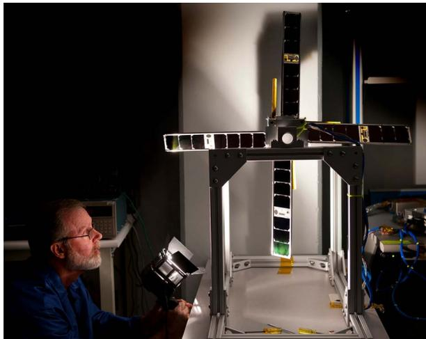
**Figure 3.** One of the MBD (Multimission Bus Demonstration) CubeSats undergoing inspection at APL. These shoebox-size satellites demonstrated that small satellites can get into orbit inexpensively and be tough enough for critical military and intelligence applications.
