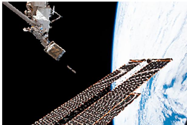
**Figure 5.** CAT (CubeSat Assessment and Test) being deployed from the ISS. Each of the two CubeSats in this APL-led flight demonstration carries a communications payload that was integrated by APL.
