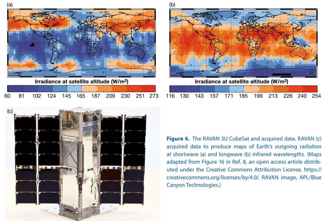
**Figure 4.** The RAVAN 3U CubeSat and acquired data. RAVAN (c) acquired data to produce maps of Earth's outgoing radiation at shortwave (a) and longwave (b) infrared wavelengths. (Maps adapted from Figure 16 in Ref. 8, an open access article distributed under the Creative Commons Attribution License, <https://creativecommons.org/licenses/by/4.0/>. RAVAN image, APL/Blue Canyon Technologies.)
