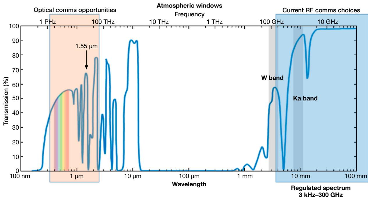
**Figure 1.** Focus areas of today's communications improvement programs. The optical (orange) part of the spectrum provides options to expand communications capability outside the RF (blue) regulated part of the spectrum.
