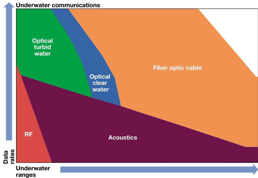
**Figure 4.** Physical limits of current underwater communications capabilities. Modalities suitable for underwater use are typically limited in either bandwidth or range, so the right set of phenomena must be chosen for the desired communication.
