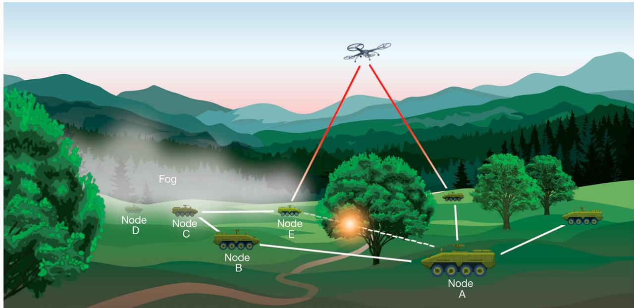
**Figure 5.** The topology control problem in FSO networking. Suppose node A has two optical transceiver heads but has line-of-sight visibility to nodes B, C, and D. To which two nodes should node A point? Node A's choice must be coupled with the choices of the other nodes since optical receivers and transmitters must be aligned.
