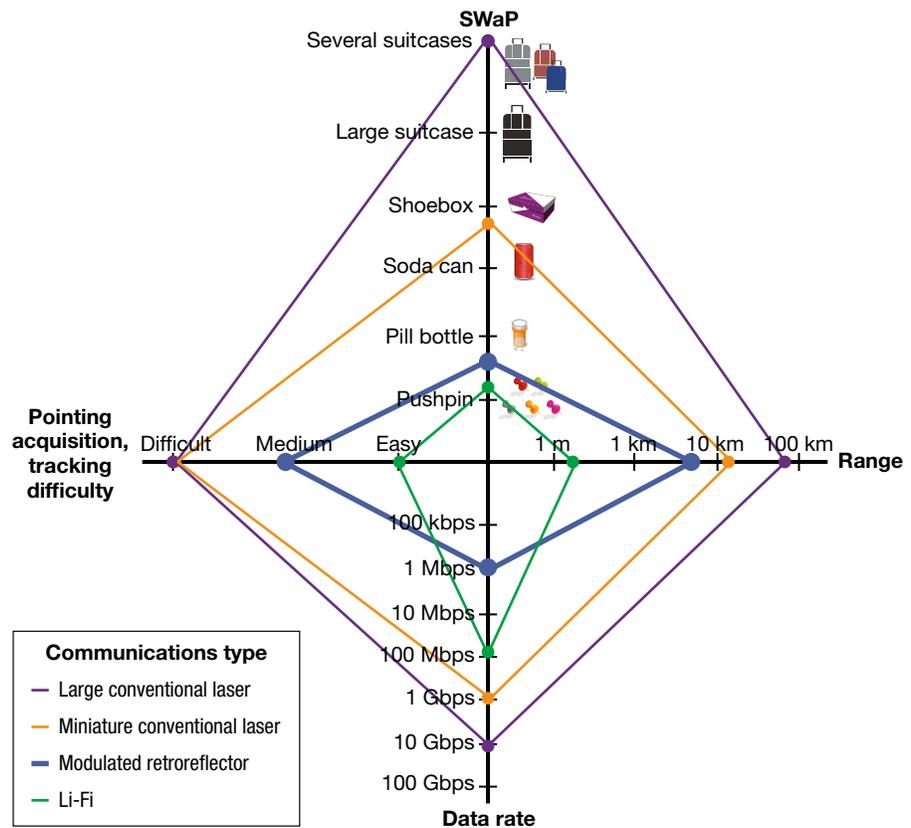
**Figure 3.** Advantages of using an MRR. The MRR is substantially smaller than a laser terminal, requires very little power, and offers a large acceptance angle that makes it much easier to align and establish a link compared with conventional laser terminals.
