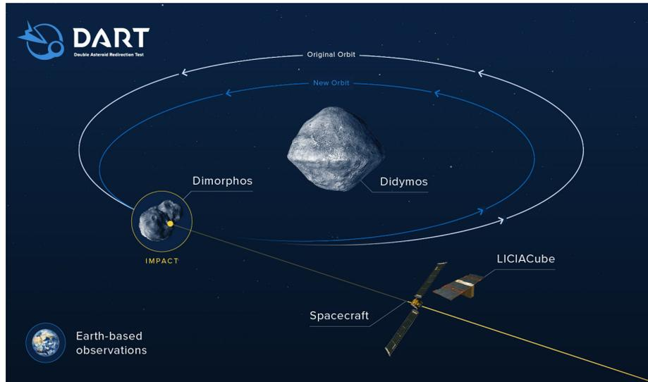
**Figure 6.** Schematic of the DART mission. This illustration shows the impact on the moonlet of asteroid (65803) Didymos. Post-impact observations from Earth-based optical telescopes and planetary radar would, in turn, measure the change in the moonlet's orbit about the parent body. (NASA/APL.)
