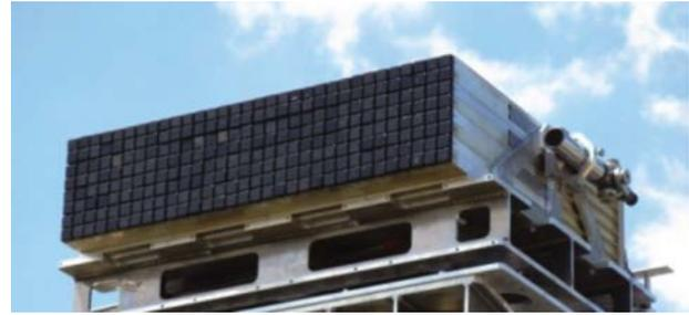
Figure 3. AUSPAR element-level digital array under test.
