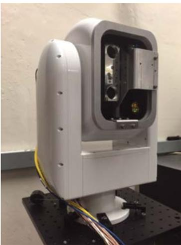
Figure 20. APL FSO terminal prototype.
