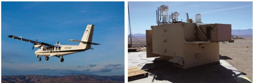
**Figure 18.** FOENEX test aircraft with two optical and one RF aperture and ground station with two optical and two RF apertures.
