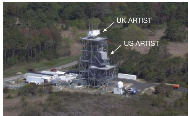
**Figure 2.** UK and US ARTIST research radars at Wallops Island, Virginia. The radars were placed at heights representative of potential locations on UK and US Navy ships.
