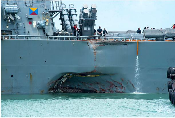
**Figure 7.** Port side of USS *John S. McCain* after a collision with an oil tanker on 21 August 2017. (U.S. Navy photo by Mass Communication Specialist 2nd Class Joshua Fulton/Released.)
