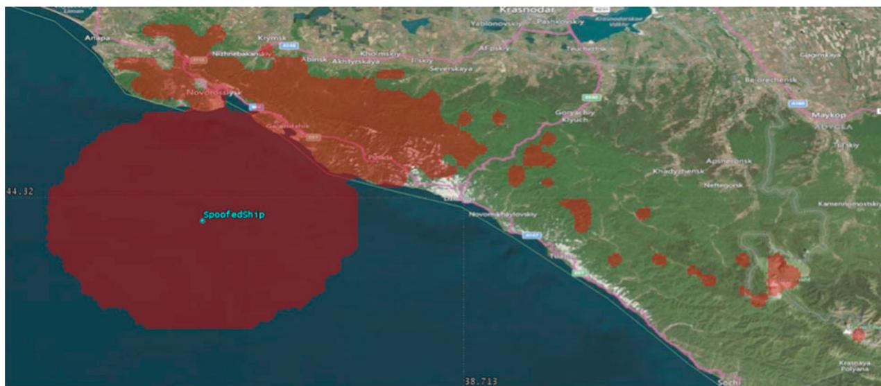
**Figure 6.** Possible spoofing source locations, based on terrain and assumed mast heights.
