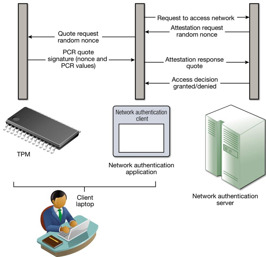
Figure 2. TPM-enabled network attestation concept showing notional requests and responses.
