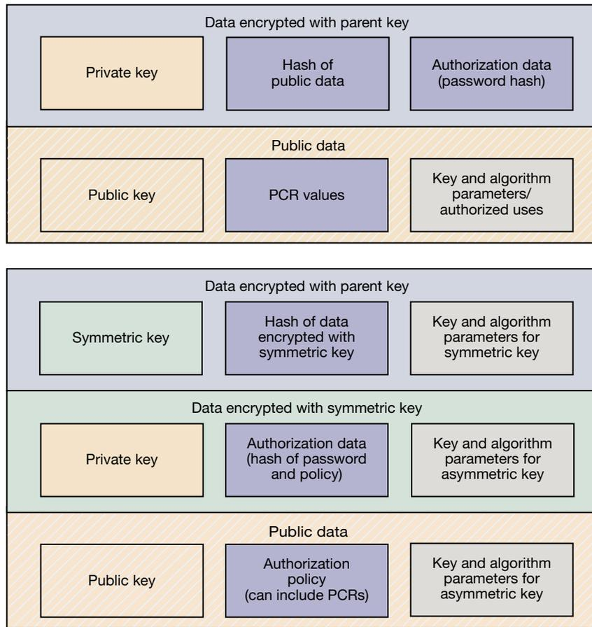
**Figure 3.** Asymmetric key structure for TPM 1.2 (top) and TPM 2.0 (bottom).
