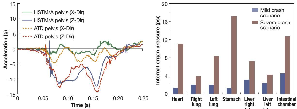
**Figure 11.** Deceleration response of the HSTM and corresponding Hybrid II (ATD) for the mild crash condition (left) and peak pressure response of the HSTM for the mild and severe crash scenarios (right).
