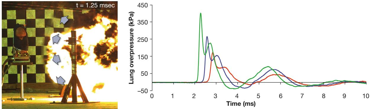
**Figure 7.** Incident shock wave approaching the HSTM during a blast test (left); upon reaching the torso surrogate, instrumentation in the lungs captures the internal overpressure response for three tests of varying charge weights (right).
