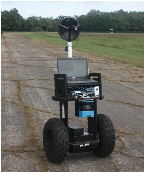
**Figure 6.** OPISR's ground vehicles were Segway RMP 200s that were fitted with lidar, electro-optic, and passive acoustic sensors.
