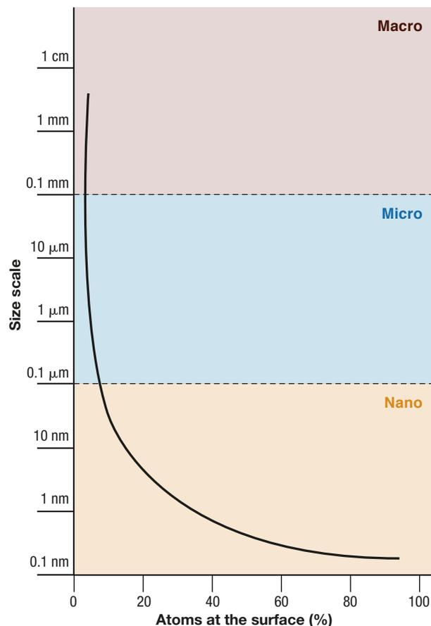
**Figure 1.** Nanoscale particles have a much larger percentage of atoms at the surface (76%) than macroscopic (millimeter-sized) particles, which have approximately 0% of atoms at the surface.<sup>11</sup>
