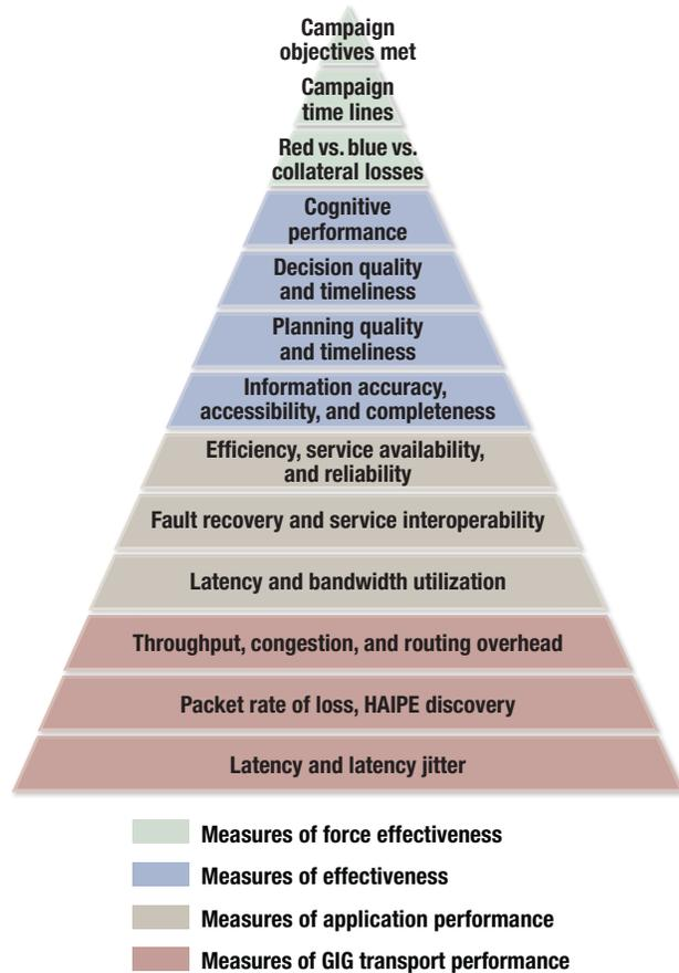
**Figure 9.** C2 metrics from effectiveness to system component performance. GIG, Global Information Grid; HAPE, High-Assurance Internet Protocol Encryptor.
