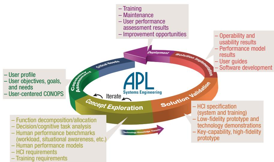
**Figure 10.** Cognitive engineering products within systems engineering. CONOPS, concept of operations; HCI, human-computer interaction.
