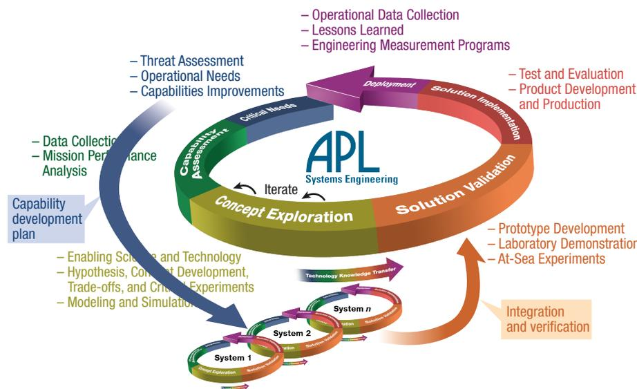
Figure 5. C2 system-of-systems engineering model.
