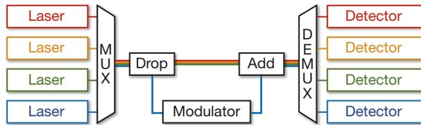
**Figure 6.** Wavelength division multiplexing using passive optical components. DEMUX, demultiplexer; MUX, multiplexer.
