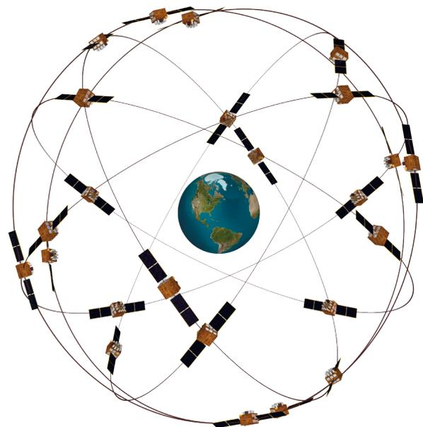
**Figure 2.** GPS satellite constellation in medium Earth orbit.
