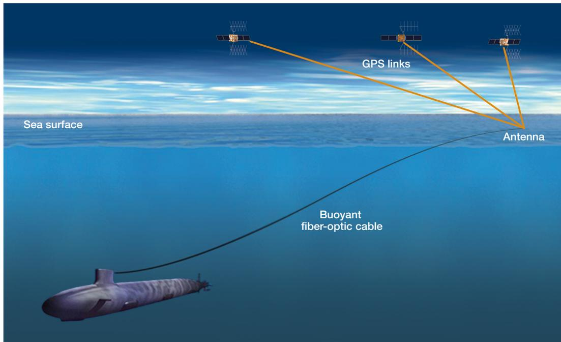
**Figure 1.** Submarine with deployed BCA for reception of GPS signals.
