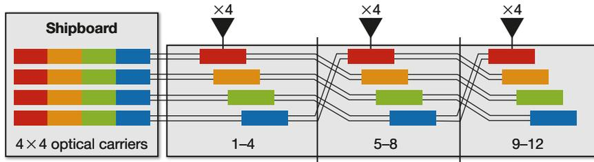
**Figure 8.** BCA with wavelength-division multiplexing and extra fiber pairs for redundancy.
