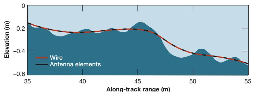
**Figure 3.** BCA floating on ocean surface. Some antenna elements are submerged or partially submerged.
