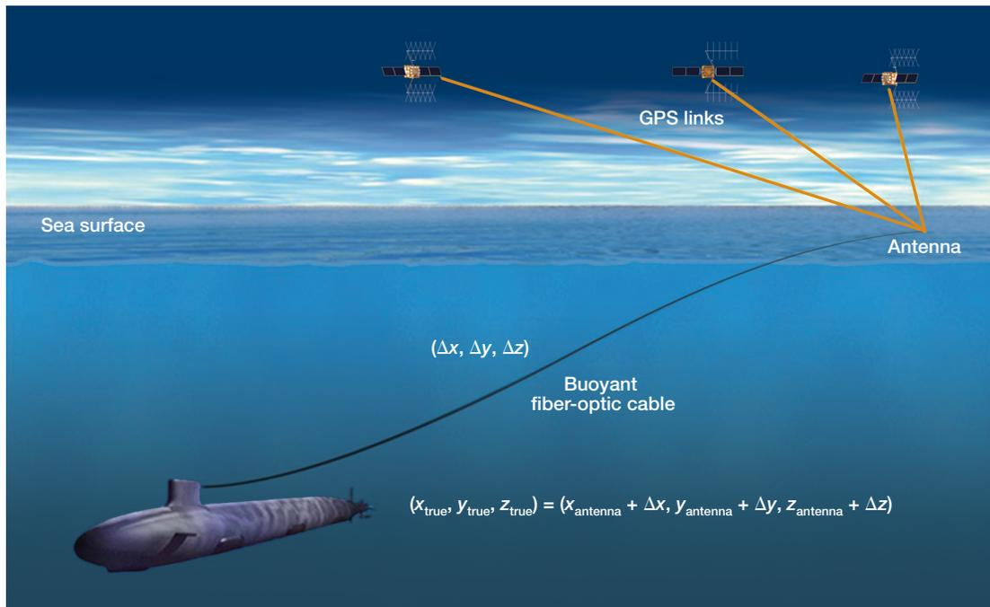
**Figure 12.** Correction for offset of GPS antenna position.
