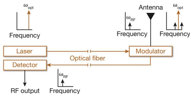
**Figure 4.** Block diagram of fiber-optic link for antenna remoting.
