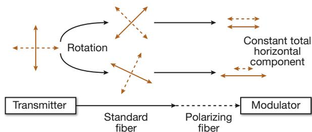
**Figure 9.** Polarization rotation of transmitted carrier components and selection of horizontal component by polarizing fiber. Even though the amount of rotation varies in the two cases shown, a total horizontal component of constant magnitude is delivered to the modulator.
