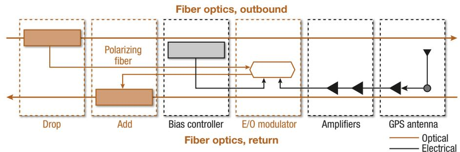
**Figure 11.** Detailed illustration of antenna node architecture.
