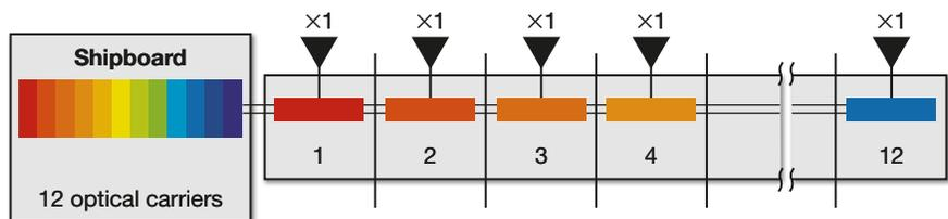
**Figure 7.** BCA with a single fiber pair. The fiber plant is a single point of failure.
