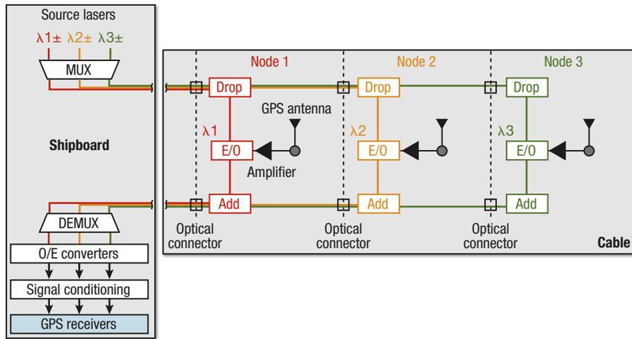
**Figure 10.** Block diagram of BCA optical network. A single fiber pair is shown for clarity. The actual network consists of four such fiber pairs with a staggered wavelength plan. E/O, electrical-to-optical conversion; O/E, optical-to-electrical conversion.
