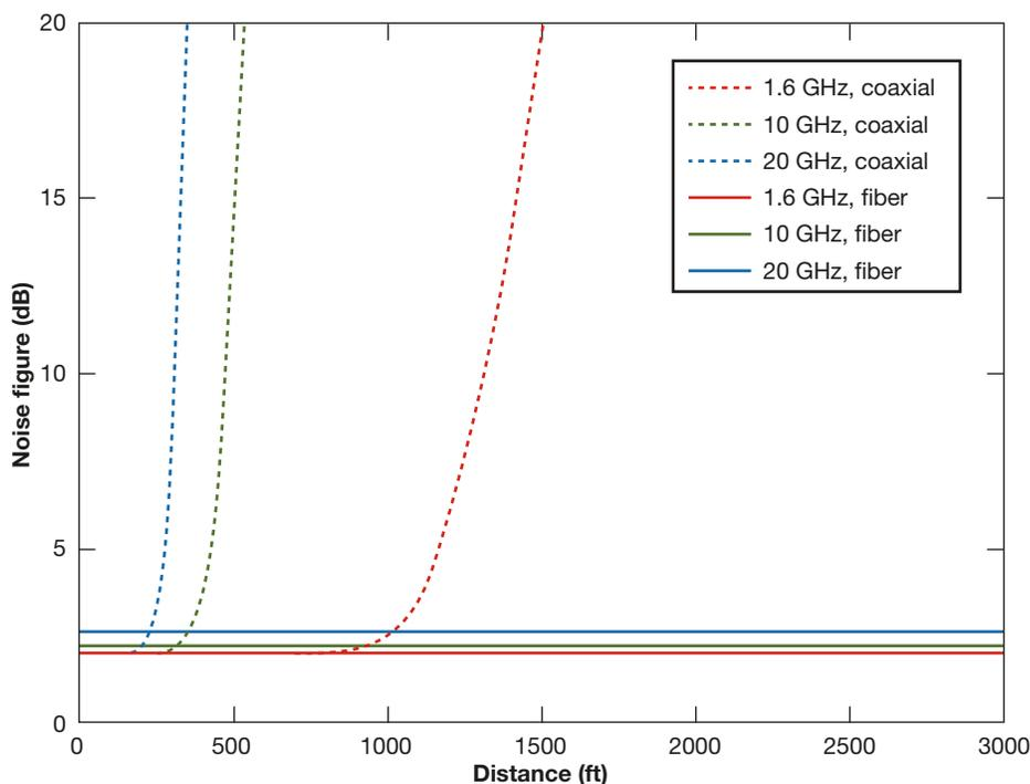
**Figure 5.** Noise figure comparison between optical fiber and coaxial cable at frequencies of 1.6, 10, and 20 GHz.
