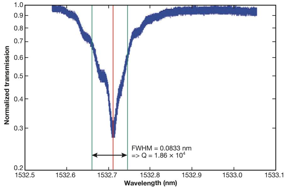
**Figure 9.** Fundamental mode resonance of a disc resonator. Typical transmission spectrum through a tapered optical fiber in contact with a ring resonator. The dip occurs when the ring diameter is an integer number of optical wavelengths. The resonance dip only drops all the way to zero if the coupling exactly matches losses in the resonator. In this case, the fiber is in contact (overcoupled) with the resonator. FWHM, full width at half maximum.
