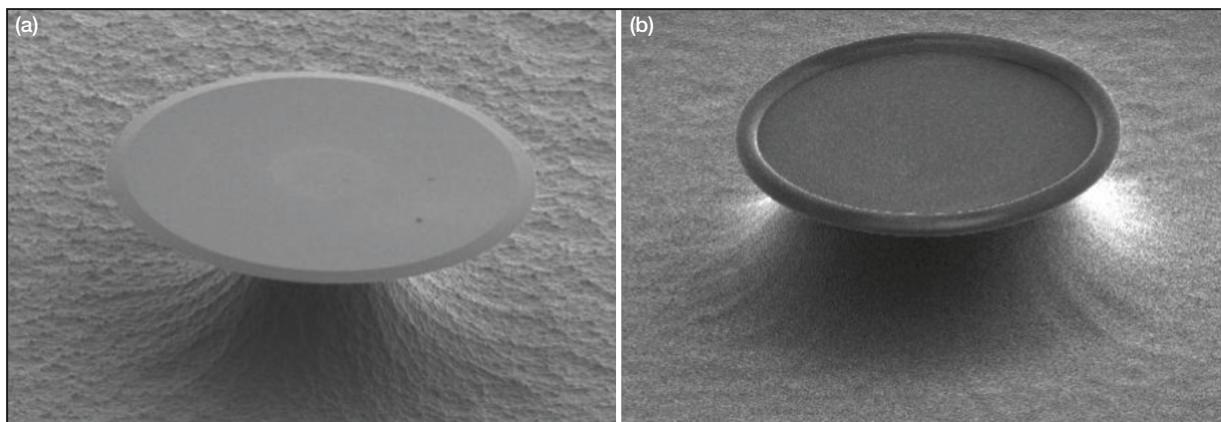
**Figure 8.** The resonant structures for the Zeno devices can be thin silica discs (a) or toroids (b). The toroids are fabricated by partially melting a disc using a  $\text{CO}_2$  laser reflow process.
