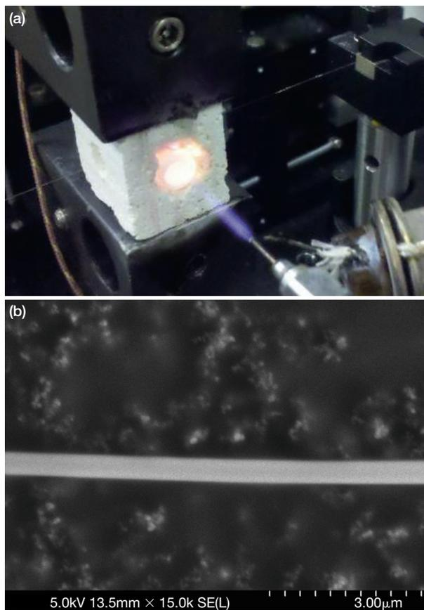
**Figure 10.** By using a homemade furnace (a) and motorized micrometers, we can pull tapered fibers with minimum diameters below  $1\ \mu\text{m}$  (b).
