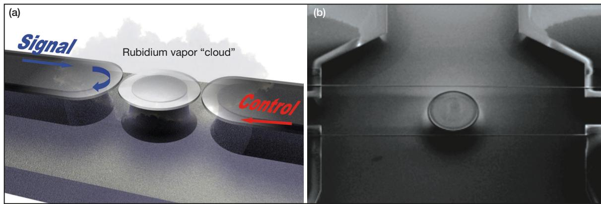
**Figure 7.** (a) Zeno effect microdevice concept, showing all features on one integrated chip. (b) Experimental Zeno switch prototype using tapered optical fibers to couple to a microtoroid.
