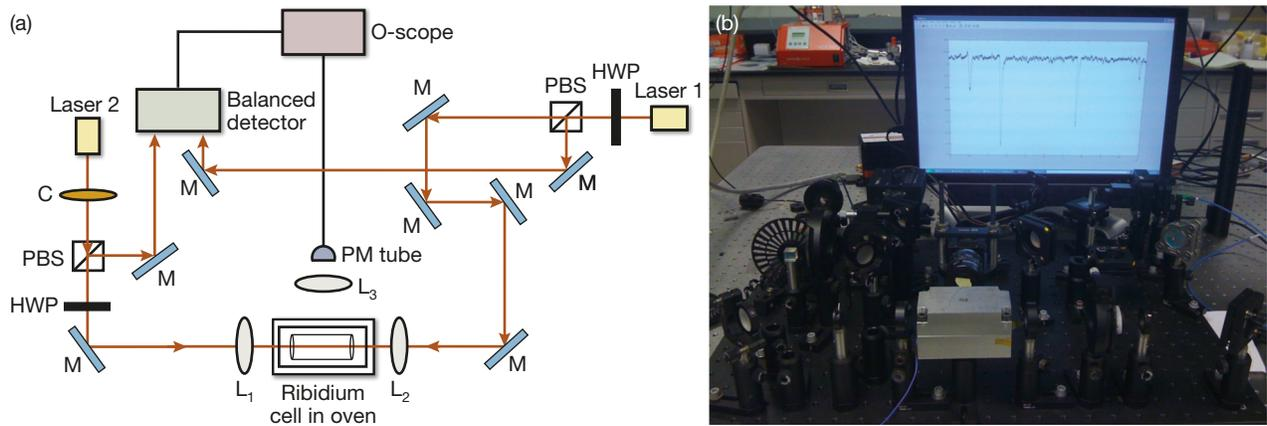
**Figure 12.** (a) Diagram of TPA setup. C, chopper; HWP, half-wave plate; M, mirror;  $L_1$ ,  $L_2$ , lens  $f = 60$  mm;  $L_3$ , lens  $f = 40$  mm; O-scope, oscilloscope; PM tube, photo-multiplier tube. (b) Actual TPA setup.
