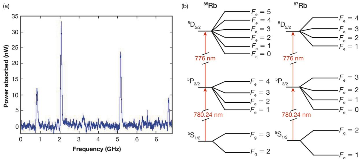
**Figure 13.** (a) TPA spectroscopic data acquired by sweeping the frequency of laser 2 with respect to laser 1. The four peaks correspond to the rubidium ground-state hyperfine levels, which can be seen in the energy level diagram (b).
