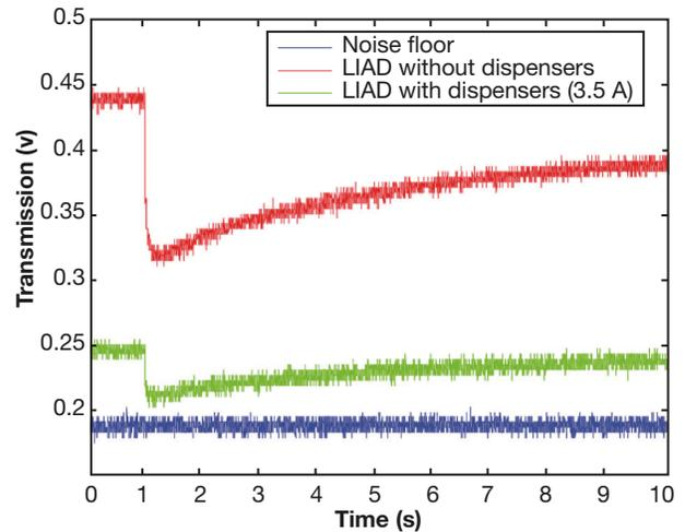
**Figure 16.** Preliminary LIAD test results showing atomic desorption decreasing transmission through the glass cell.
