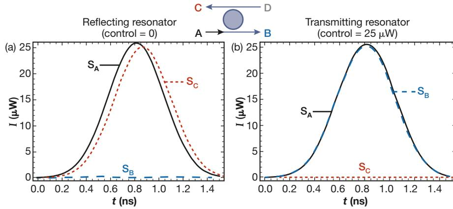
**Figure 5.** Dynamic simulation result showing low-loss optical switching. (a) With the control off, the output signal ( $S_C$ ) is a slightly delayed and attenuated version of the input,  $S_A$ ; (b) with the control on, the output signal ( $S_B$ ) follows the input with very little loss. These results highlight the counterintuitive nature of the Zeno effect, because the losses when TPA can occur (control on) are actually less than when it cannot.
