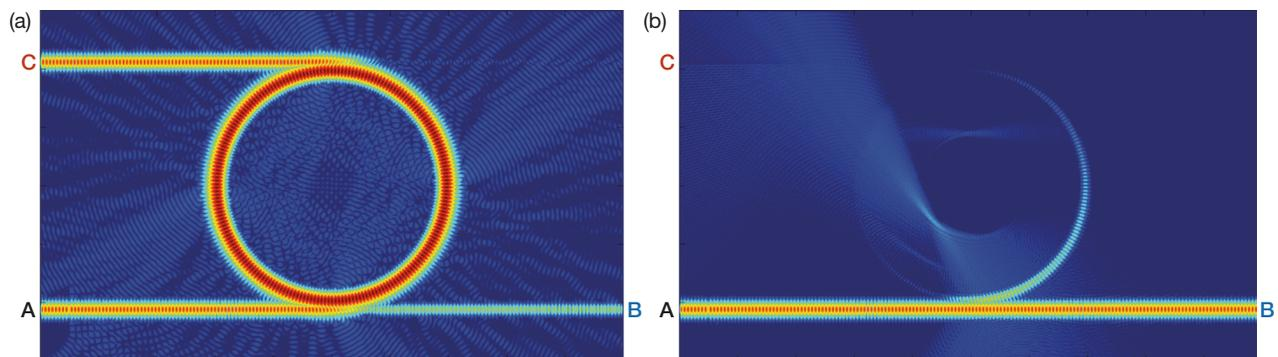
**Figure 4.** Numerical simulation of the optical switch with the control off (a) and on (b). In both panels, the source enters the switch from the lower left (mode A), and the control field is not shown in either panel. With the control off, the intensity in the resonator grows and the signal exits at the upper left (C). With the control-on energy entering, the ring is dissipated and the signal exits the lower right. Color scale is relative intensity in decibels.
