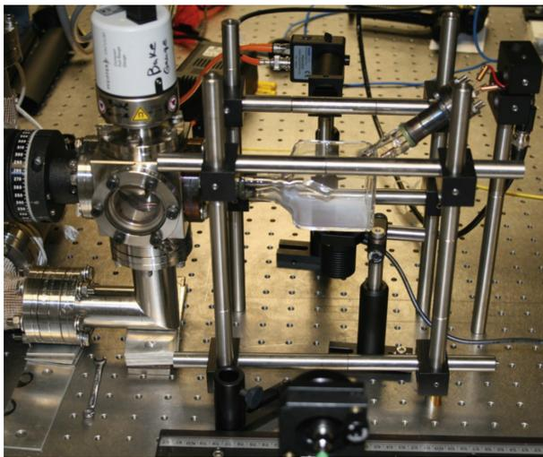
**Figure 15.** APL glass cell coated with rubidium atoms and attached to the vacuum system.
