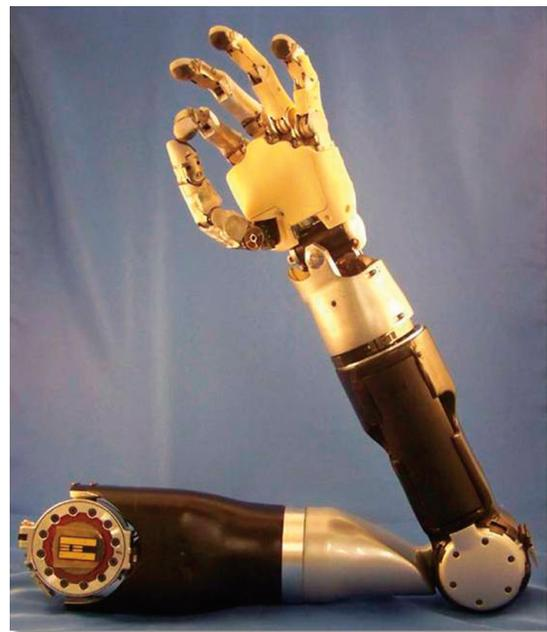
**Figure 1.** This final prototype of the MPL, successfully demonstrated to DARPA in December 2009, offers 22 degrees of freedom.
