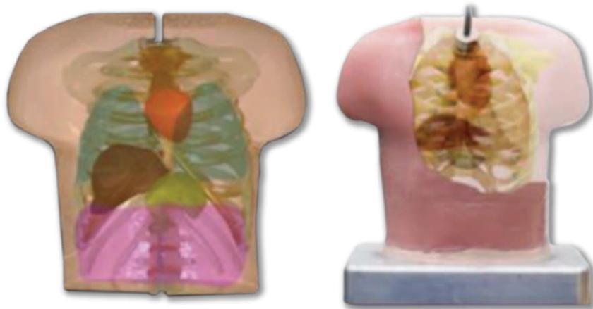
**Figure 9.** Computer solid model (left) and actual human surrogate torso model (right).
