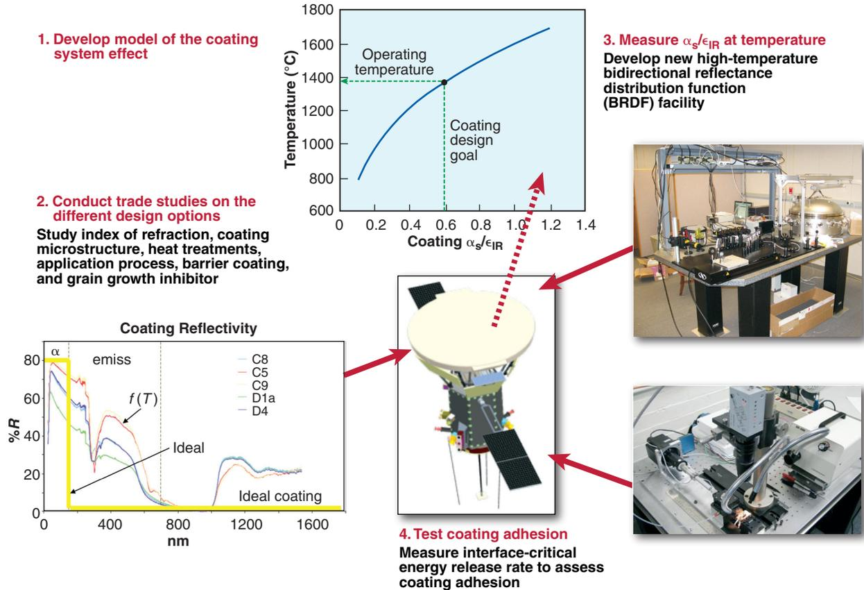
**Figure 2.** Development of candidate coating technologies, along with the measurement techniques used to assess both their optical properties and their adhesion.
