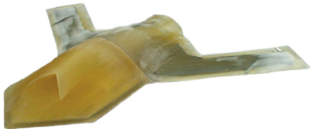
Figure 1. Air Force unmanned combat air vehicle RP wind-tunnel model constructed by APL.
