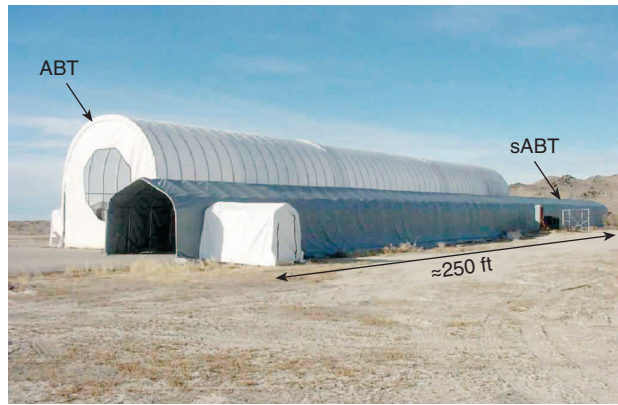
Figure 2. Photograph of the Ambient Breeze Tunnel (ABT) and stand-off Ambient Breeze Tunnel (sABT) at Dugway Proving Ground.
