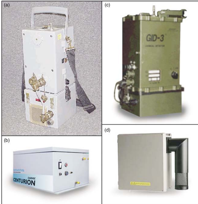
Figure 5. A variety of commercial chemical sensors rely on ion mobility spectrometry, surface acoustic waves, and electrochemical reaction for detection. They offer reliability, orthogonality, sensitivity, and specificity: (a) Shipboard Automated Chemical Agent Detection Alarm (ACADA), (b) Centurion field tester, (c) Graseby Ion Detector (GID-3), and (d) CW Sentry Plus.
