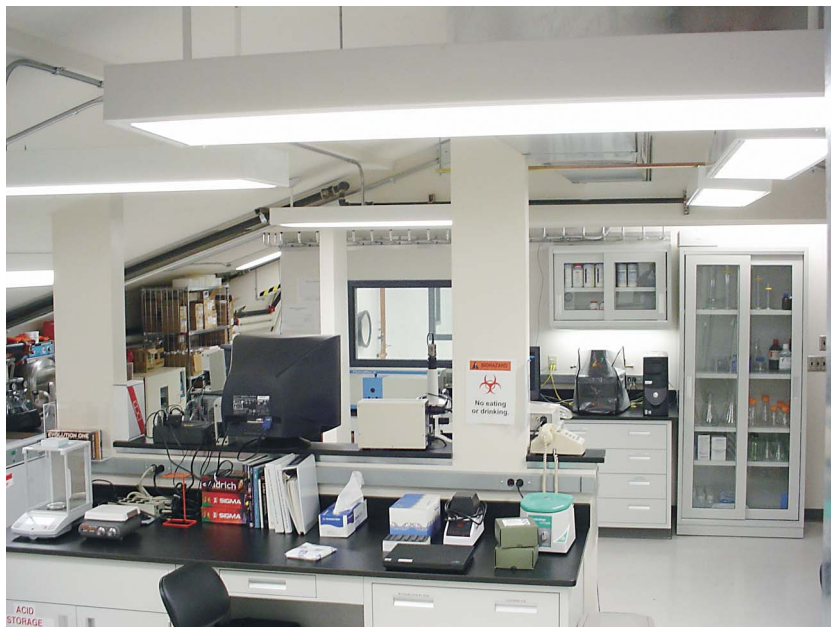
Figure 4. Biosafety Level 2 portion of the CBTEC. An observation window looking into the aerosol chamber section of the facility is shown in the center of the photograph.
