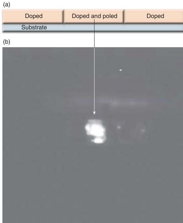
**Figure 14.** Electro-optic lightguide formed using chromophore-doped polyimide. In the poled film, the chromophores have been aligned under a strong electric field. (a) Schematic cross section of a guide. (b) Light containment achieved by an experimental version of a guide fabricated at APL.
