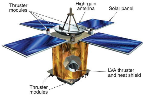
**Figure 1.** NEAR spacecraft flight configuration (LVA = large velocity adjust).
