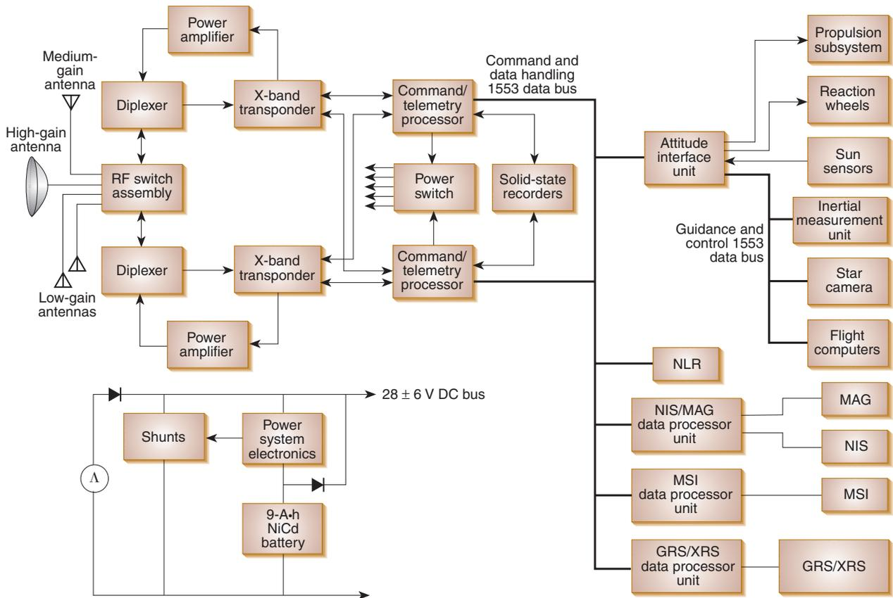
**Figure 2.** NEAR system block diagram (GRS = Gamma-Ray Spectrometer, MAG = Magnetometer, MSI = Multi-Spectral Imager, NIS = Near-Infrared Spectrograph, NLR = NEAR Laser Rangefinder, XRS = X-Ray Spectrometer).
