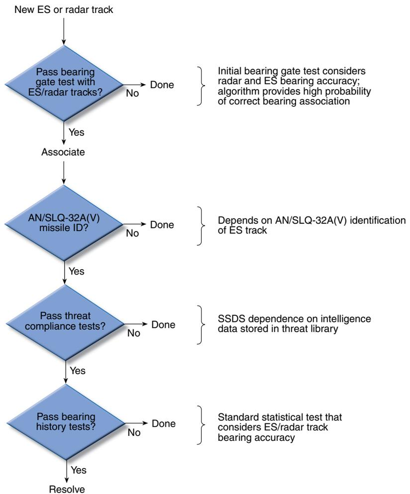
**Figure 1.** Simplified SSDS ES track/radar track association resolution thread. If more than one ES/radar track passes the test, an ambiguous marking will occur.
