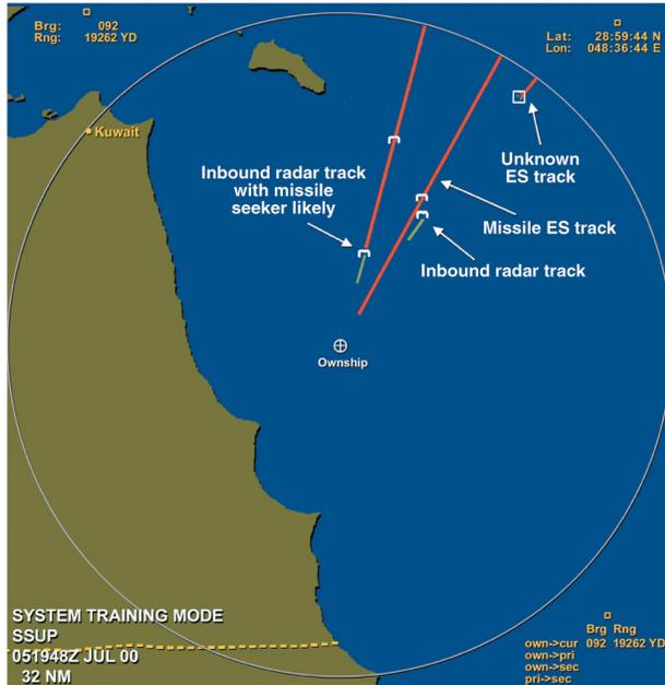
**Figure 3.** This SSUSP Sensor Supervisor PPI display shows two inbound radar tracks and three ES tracks. One ES track is unknown, one is identified as a missile but is not associated with high confidence to any radar track, and the third is identified as a missile seeker and is automatically associated with high confidence to the target to which it belongs.
