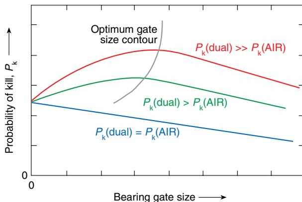
**Figure 2.** The optimum gate size depends on the exact difference between RAM modes. An appropriate bearing gate size was selected for the SSDS Mk 1 on LSD 41 class ships given the characteristics of the near-term threat, the reporting characteristics of the AN/SLQ-32A(V), and the performance difference between RAM modes.
