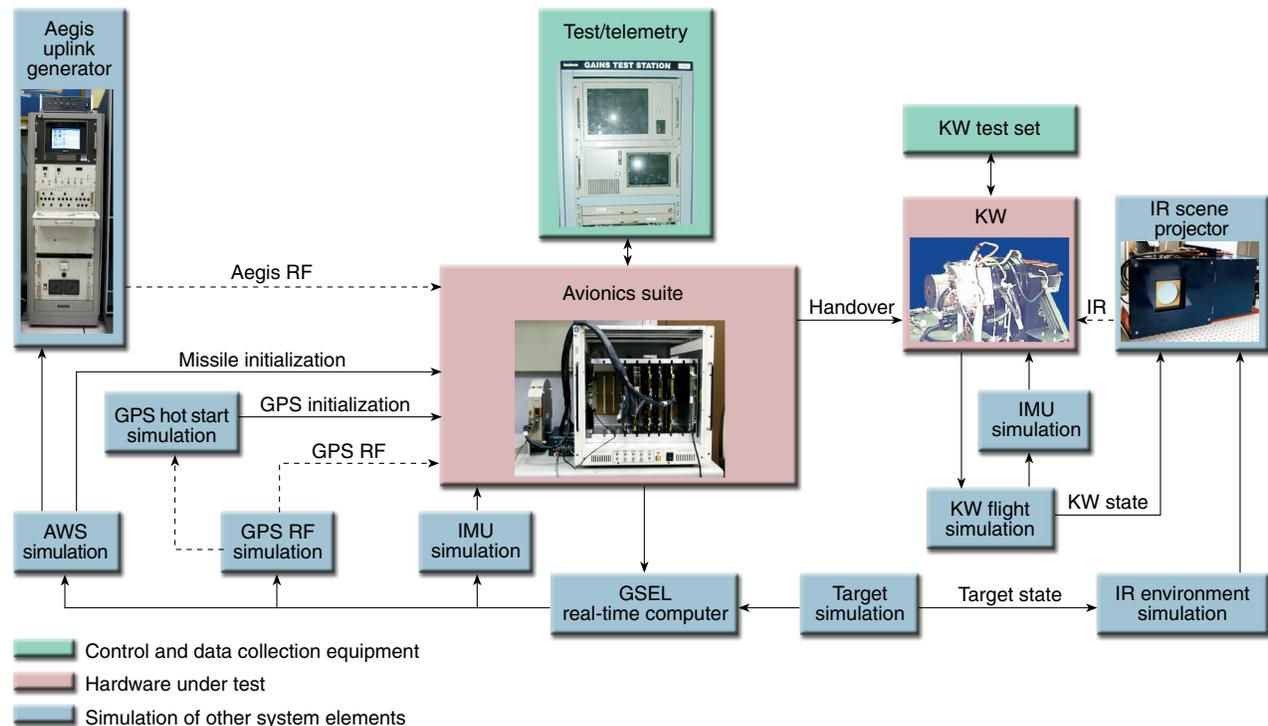
Figure 6. GSEL test configuration.
