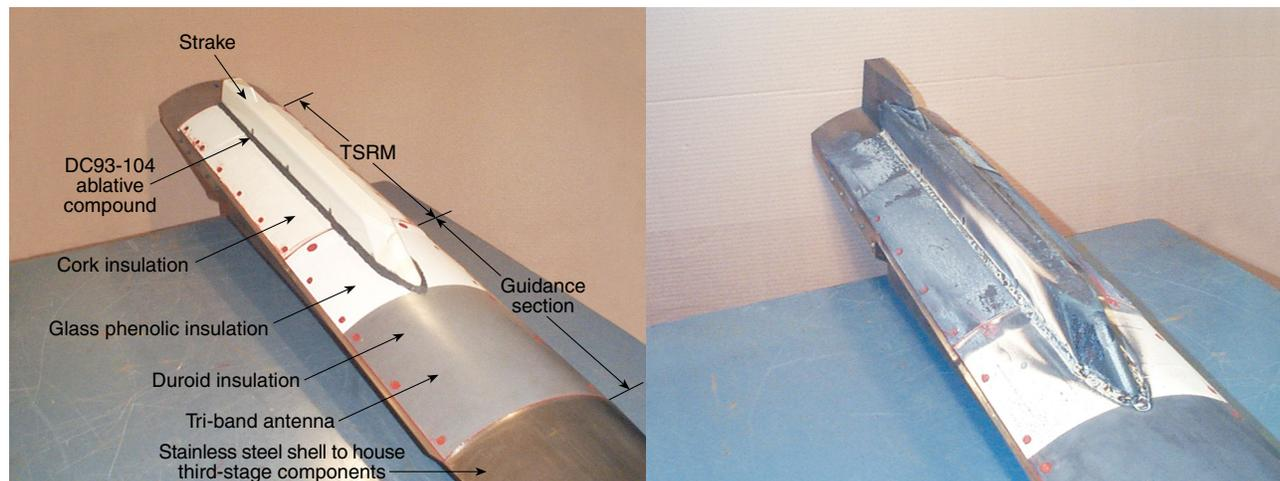
**Figure 14.** Before (left) and after (right) photographs of the TSRM test sample.
