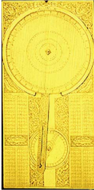
Instrument derived from studies of Galileo to determine the orbits and periods of satellites of Jupiter
