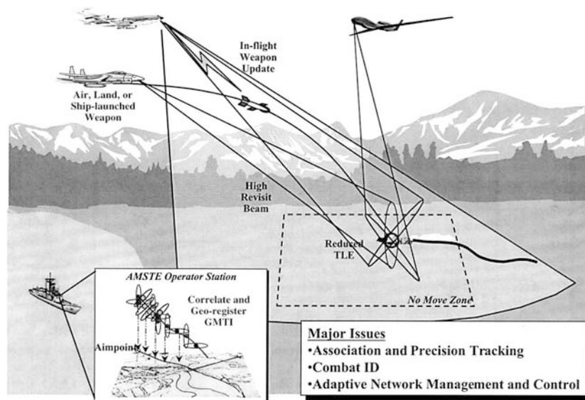
**Figure 3.** The Affordable Moving Surface Target Engagement (AMSTE) System concept (GMTI = ground moving target indicator, TLE = target localization envelope).
