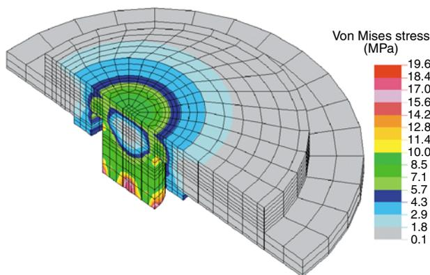
**Figure 8.** Finite-element analysis of a high-power transistor package design showing a concentration of stress at the center ring caused by the brazing of pure copper. Stress was alleviated by changing material to a copper alloy, which retains greater yield strength after brazing.
