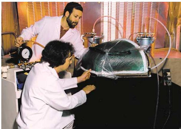
**Figure 2.** Low-cost composite fabrication technique (SCRIMP<sup>®</sup>) being used to produce hydrodynamic submarine fairings to protect sensors during operational trials for the Navy’s SCAMP Program. The APL-prepared fairings were the first known demonstration of this processing technology at sea.
