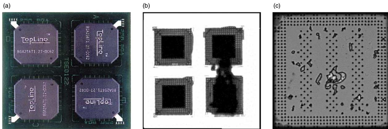
**Figure 7.** Inspection and part screening of microelectronics using C-mode scanning acoustic microscopy (CSAM) with TSD's upgraded SONIX HS-1000 unit: (a) image of a ball grid array, an example of a high-density interconnect technology, (b) a CSAM through-transmission image of printed circuit board delamination, and (c) CSAM reflection image of a flip chip showing underfill flaws.
