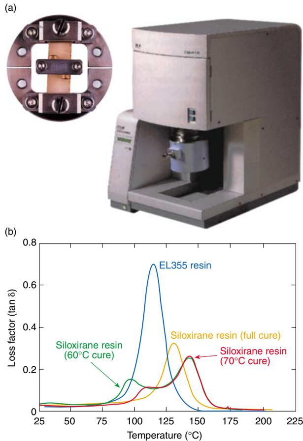
**Figure 6.** Complete characterization of viscoelastic materials, such as new polymeric resin systems, requires techniques like dynamic mechanical analysis (DMA). TSD's newly acquired Seiko DMS6100 unit (a) has a three-point flexure sample and fixture. Representative data on two high-performance resin systems are presented in (b).
