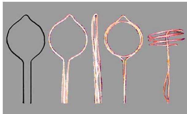
**Figure 3.** A superelastic shape-memory alloy (SMA) being considered for antennas for an MRI-guided, catheter-deployed biomedical device. Center coil is shown in retracted position (leftmost coil represents an uncoated SMA, remainder are copper plated; multiturn coils are shown at right).
