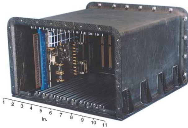
**Figure 4.** The Composite Card Cage Enclosure, also called the Integrated Electronics Module, made predominantly of carbon-fiber-reinforced composites.
