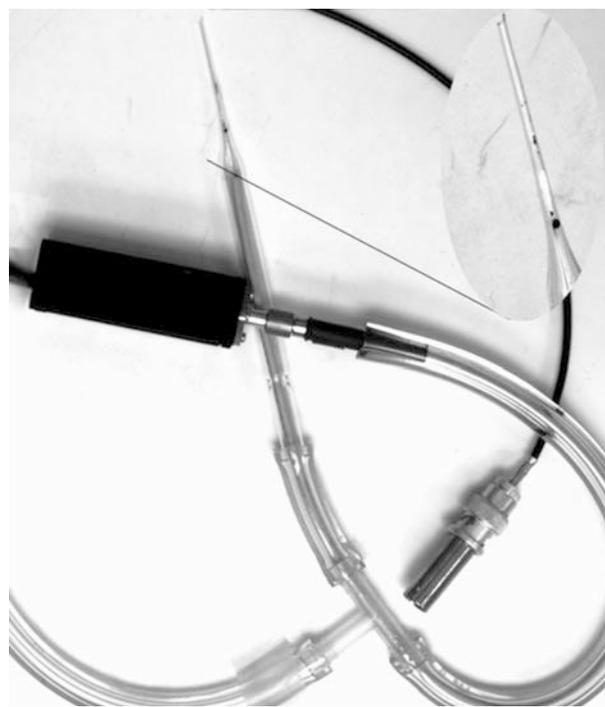
**Figure 1.** A prototype explosives detection sensor using molecularly imprinted polymer synthesis technology developed at APL.
