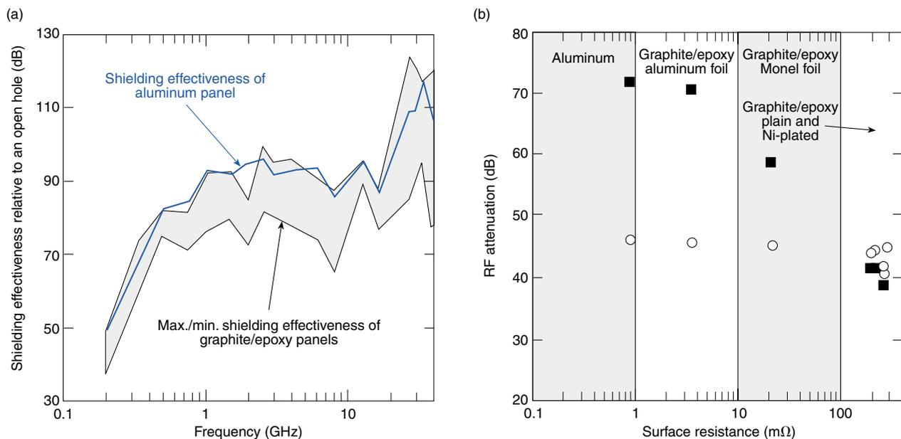
**Figure 5.** Comparison of results for aluminum to surface-modified composite panels for (a) EMI shielding effectiveness and (b) surface resistance (squares and circles are 1 and 25 MHz RF frequency, respectively). The materials were evaluated for potential use in a spacecraft electronic enclosure.
