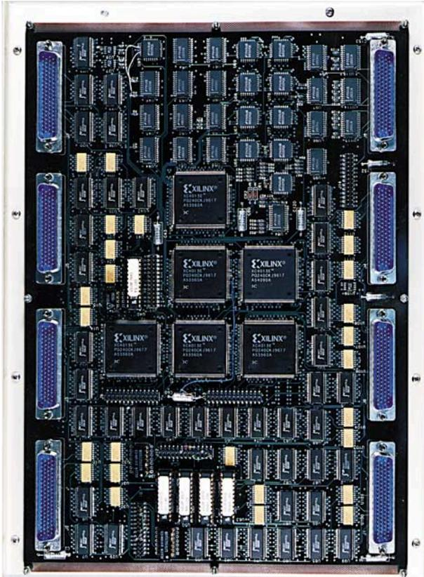
**Figure 9.** High-density PWB developed for the TRIAGE Program. This radar data collection board contains 10 circuit layers, 4883 vias, and 422 components, with 6052 internal component connections and 624 input/output pins. This single board replaced the five boards used in a previous system.
