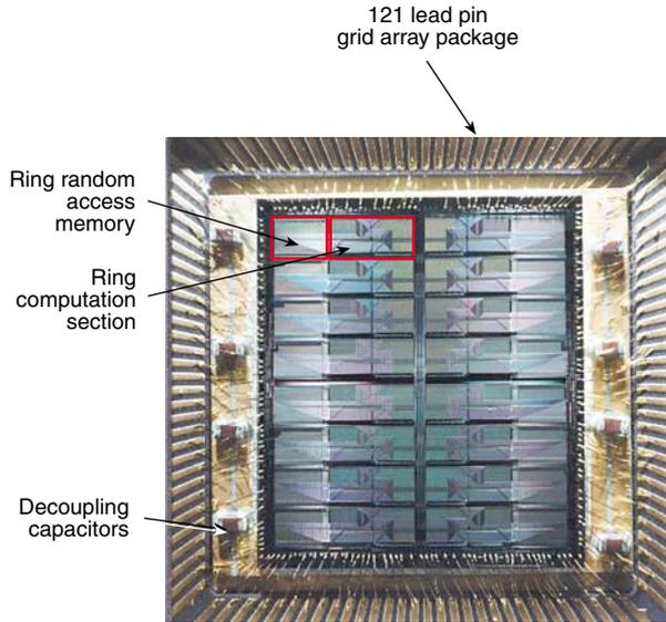
**Figure 3.** DIMUS IC chip custom-designed in the EDF. DIMUS uses CMOS technology and was designed with APL's MAGIC, IRSIM, and ModelSim software and fabricated through the MOSIS network. It contains 2 million transistors and uses 0.8- $\mu\text{m}$  design rules.
