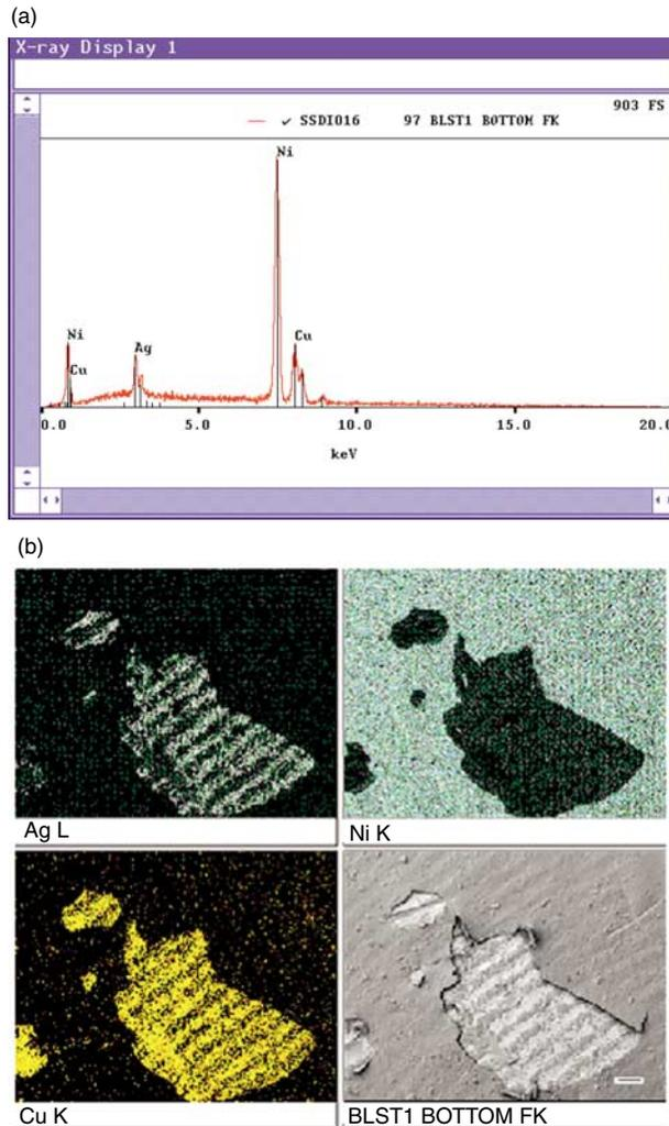
**Figure 13.** Energy-dispersive X-ray spectrum (a) and dot maps (b) of a blister on the nickel-coated copper case of a high-powered electronic switch. Dot maps shown are for silver, nickel, copper, and a scanning electron micrograph of the region.
