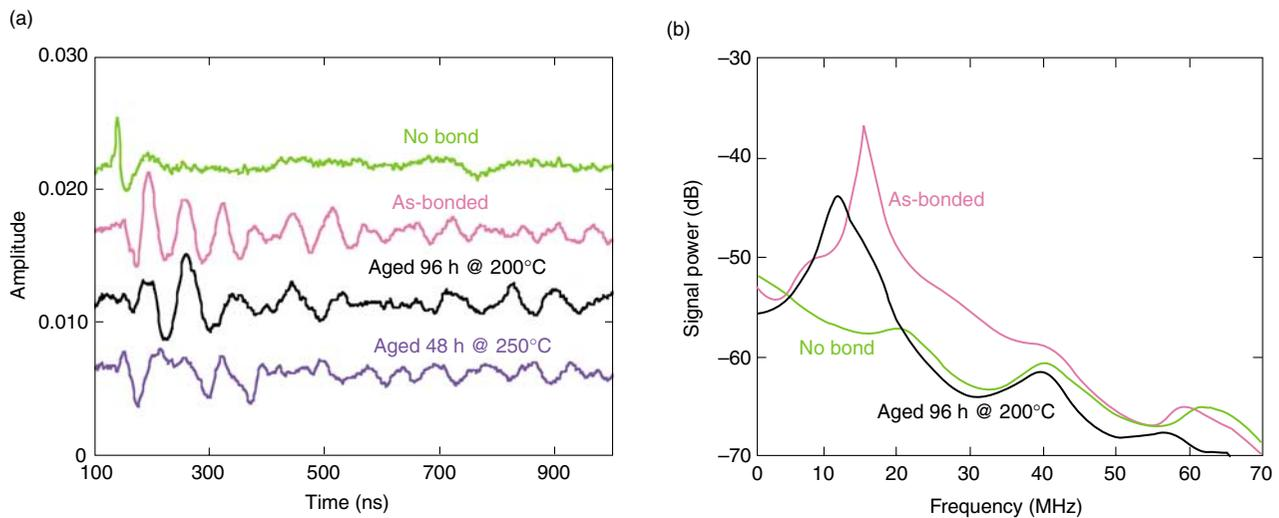
**Figure 15.** (a) Surface amplitude versus time as the wave train passes the silicon surface position detector as measured for differently aged samples (offset for clarity). (b) Example of the power spectral density numerically extracted from the time domain data in (a).
