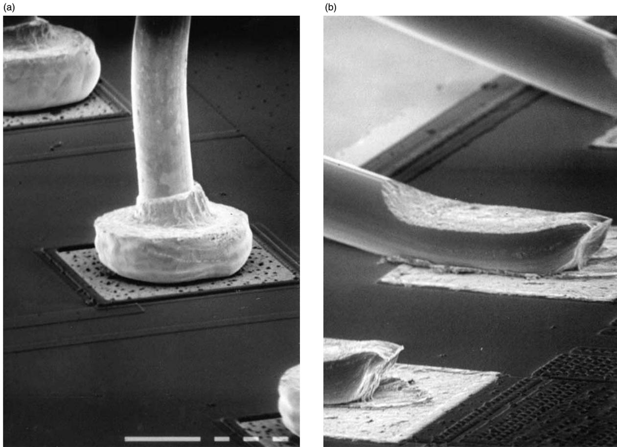
**Figure 14.** Microelectronic ball (a) and wedge (b) wirebonds.
