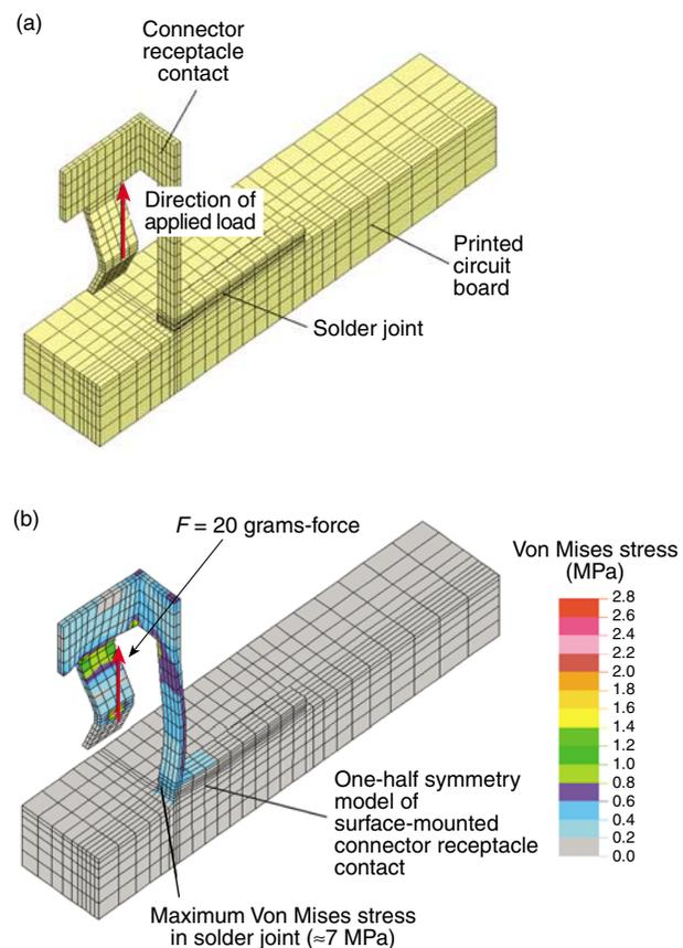
**Figure 8.** Finite-element analysis of a Minitек surface-mount connector used on the TIMED spacecraft. (a) One-half symmetry finite-element model of a single Minitек surface-mount receptacle contact. (b) Von Mises stress contours for the Minitек connector.
