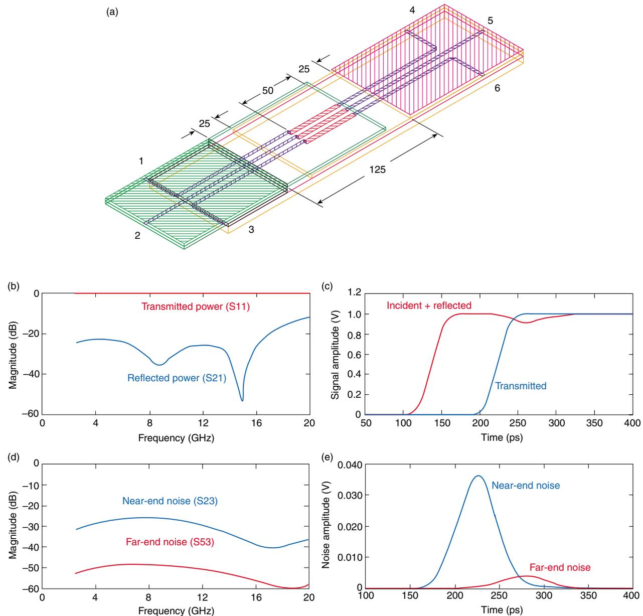
**Figure 6.** High-speed stripline cables to MCM-soldered interconnection. (a) Physical layout (dimensions in mils; ports labeled 1 to 6). (b) S-parameter data for cable to MCM-soldered interconnection. (c) Signal transmission/reflection analysis (9% reflected noise). (d) Cross-talk analysis S-parameter data for coupled three-line model for cable to MCM-soldered interconnection. (e) Cross-talk noise analysis (3.7% near-end noise, <1% far-end noise).
