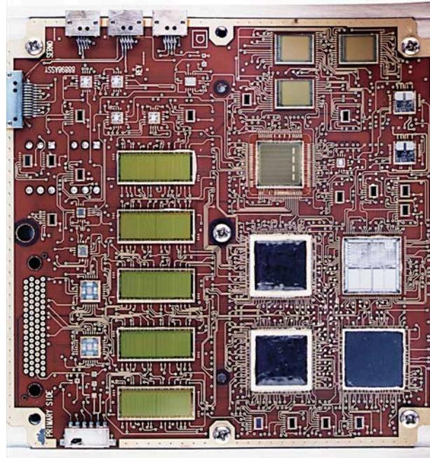
**Figure 10.** COB substrate containing blind and staggered vias. This  $12.3 \times 12.3$  cm board is being used for the palm-sized Command and Data Handling System.<sup>19</sup>
