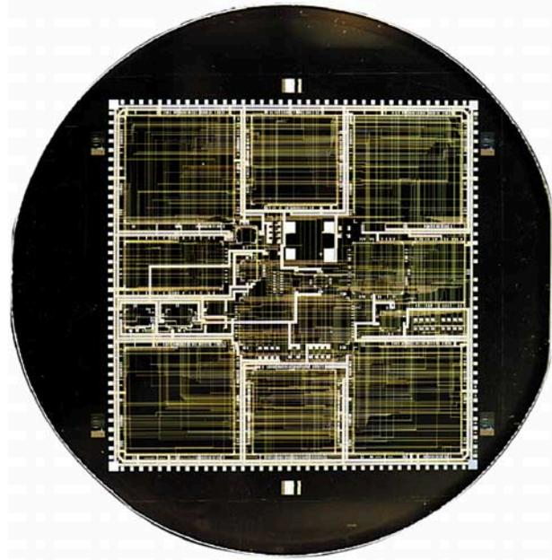
**Figure 4.** Thin film multilayer MCM. The substrate was fabricated using EDF's copper/polyimide MCM-D technology. It is about 13 cm<sup>2</sup> and contains three buried layers of circuitry. The assembled unit has 16 chips and over 1200 wirebonds.
