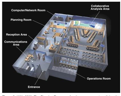
Figure 3. WAL 2000. The Planning Room can function as a separate collaborative meeting area with a stand-alone 12-workstation ESS System, or it can be used in conjunction with activities in the Collaborative Analysis Area. The main area has been enhanced to include a 50-station ESS System, 50-seat observer gallery, large-screen displays, video teleconferencing, information network access, models and simulations, and scenario and parametric databases.
