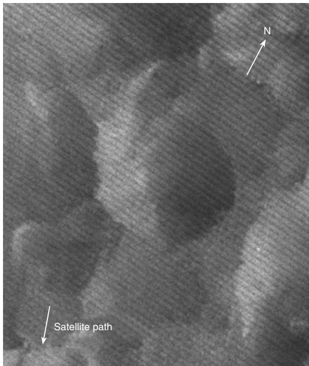
**Figure 2.** Radarsat-1 ScanSAR wide B image of a round storm cell (© Canadian Space Agency [CSA], 1998).
