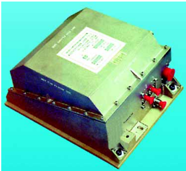
Figure 3. Trident II (D5) translator. This is an RCA production D5 translator on a test fixture. This model translator has flown in all D5 test missiles. The base dimensions are approximately 7.0 × 9.6 in.
