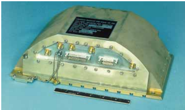
Figure 2. Trident I (C4) translators: The two translators shown were designed to the same specifications. The base dimensions are approximately 6.5 \times 12.3 in. (a) The prototype designed at APL was subsequently used in a satellite for system demonstration and checkout activities. (b) One of the production units designed by RCA has supported C4 test flights since 1978.
