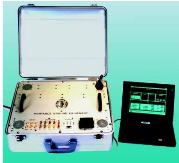
Figure 5. Extended Navy Test Bed receiver/recording equipment. The suitcase shown here with the laptop control computer includes all the hardware needed to record duplicate (for right- and left-hand circularly polarized downlink signals) full-bandwidth, dual-frequency GPS signals for more than 1000 s. The suitcase is designed to connect to the telemetry station multiplexer that distributes S-band telemetry signals to all telemetry receivers.
